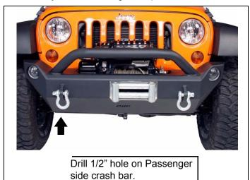
c. Install four *kit* bolts (1/2" x 1 1/4" Button Head) with large thick washer and flange nut through outer holes on bottom of bumper. (Note: Some models are not equipped with this hole. It will be necessary to mark and drill a 1/2" hole to complete step.)
