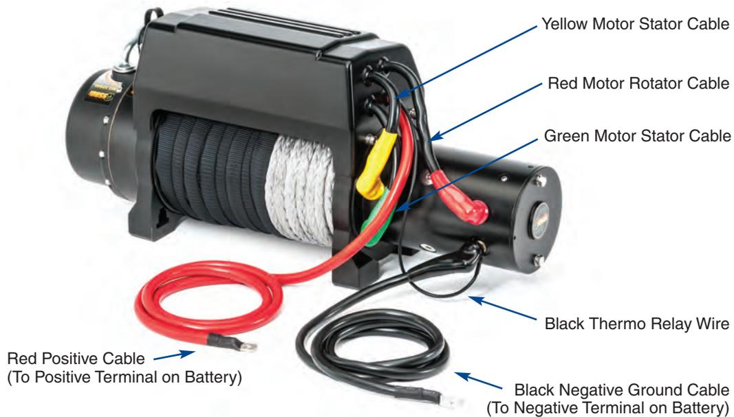
*Attach black ground cable to motor terminal and black thermo relay wire with brass bolt. Tighten brass bolt onto terminal using a 14mm wrench.*
