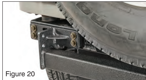
to the vehicle to 45 ft/lbs using a torque wrench. Attach the receiver hitch to the rear frame using (4) 10mm bolts, (8) 10mm Flat Washers, (4) 10mm Lock Washers (Fig 21) and (4) 10mm nuts per side. Proper bolt, washer and nut position called out in (Fig 18). Tighten these bolts/nuts to 45 ft/lbs using a Torque Wrench. Proceed to Step 3.
