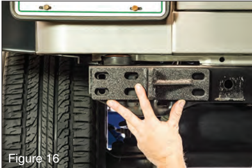
Attaching Mounting Brackets With the four 1/2" Holes drilled, the brackets/Hitch should be centered on the holes with the vertical mounting tab
