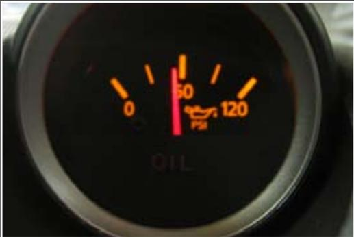
15. While engine is warming up **DO NOT** rev the engine. Double check the oil cooler lines and fittings for leaks during the warm up process.
