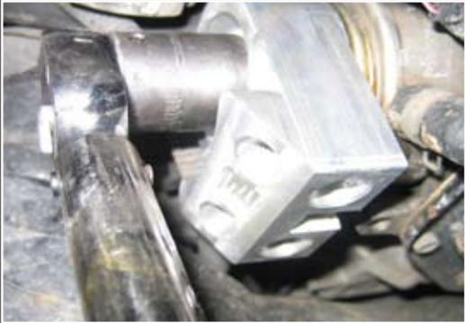
5. Install the oil block off fittings as pictured. Remember, Teflon tape is only to be used on the NPT fittings in the end of the block-off caps. Rubber o-rings should be between the block-off bolt (24mm) and the oil filter block. Torque the 24mm hex head block-off fittings to 25ft/lbs and install the 1/8in NPT pipe thread caps with Teflon tape.
