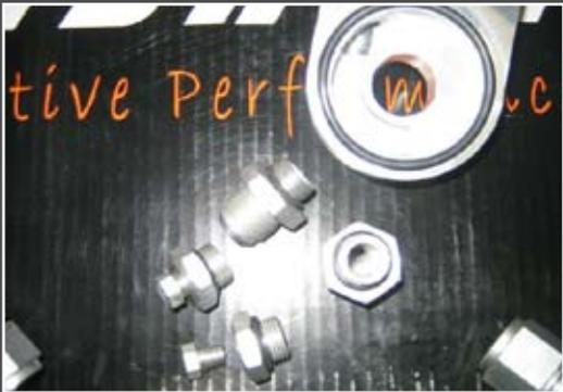
2. Locate the oil filter adapter plate fittings that came with the Mishimoto oil cooler. Use the factory oil filter to locate the correct oil filter thread for your car. Screw the fittings in as shown and make sure you use the fitting that screws into the oil filter without **ANY** play in the threading. There are 3 main thread sizes for oil filters and they are very close to each other. Take extra care to select the correct fitting. Two of these fittings will not be used.
