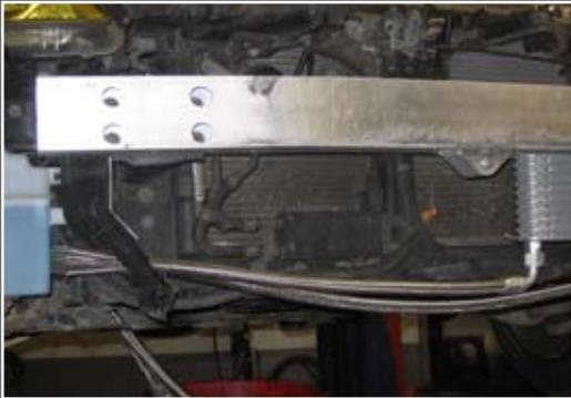
11. Attach the lines to the oil filter block. The oil cooler connections do not have to be installed on any specific port. Use a wrench to hold the fitting oil filter block and to keep it from spinning and tighten the fitting on the oil cooler line. Install the oil filter at this time. The cooler lines should be above the connection for the lower control arm. Lines that are lower than this should be re-located to prevent possible damage from road debris.
