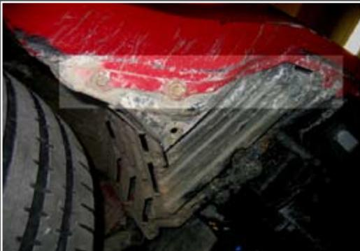
3. Peel the wheel well splash guard out from behind the front bumper near the fenders and remove the (3) 10mm head bolts inside on both sides of the front bumper. (See picture)
