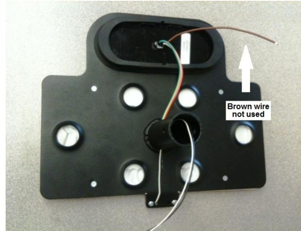
4. Next, install the rubber gasket for the 6" oblong LED brake light. Press the light into the gasket firmly until it seats completely. We are only utilizing the green (+) and white (-) wires, so the brown one can be trimmed short and taped off.
