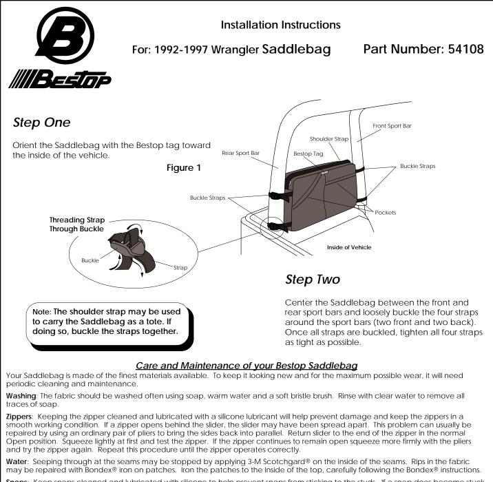
**Snaps**: Keep snaps cleaned and lubricated with silicone to help prevent snaps from sticking to the studs. If a snap does become stuck to a stud, use a screwdriver and GENTLY pry apart to prevent permanent damage to the snap or the top fabric.
