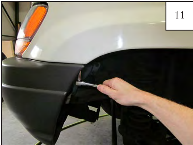
Using a 10mm socket and ratchet, remove factory screw from top of front bumper. Retain screw for re-installation.
