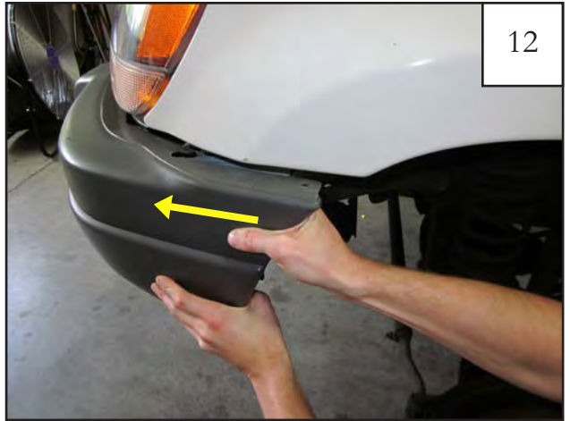
Push front bumper forward away from wheel well to release from factory installed clip in fender.
