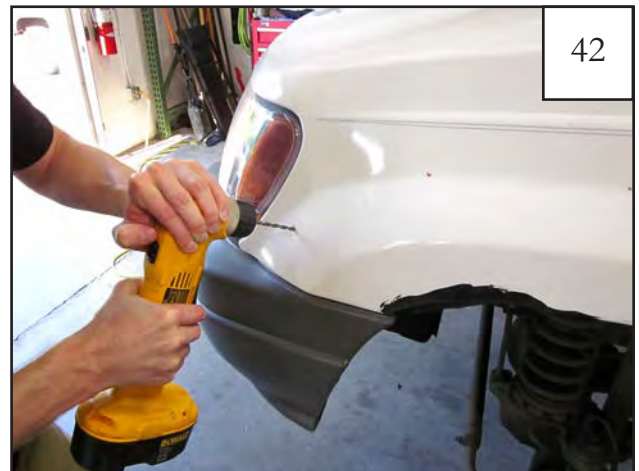
Using a 3/16" drill bit, drill holes marked in step 41.
