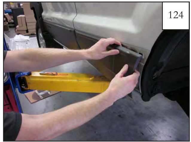
Pull firmly to remove upper factory side cladding piece from fender.
