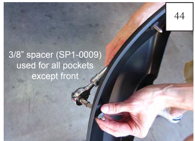
For all remaining pockets, install a #45 Torx screw (SW1-0045) through pocket hole and secure with rubber spacer ( SP1-0009 ) using supplied #45 Torx bit (SW1-0052). Drive screw into spacer until tight. Repeat for all remaining pockets.
