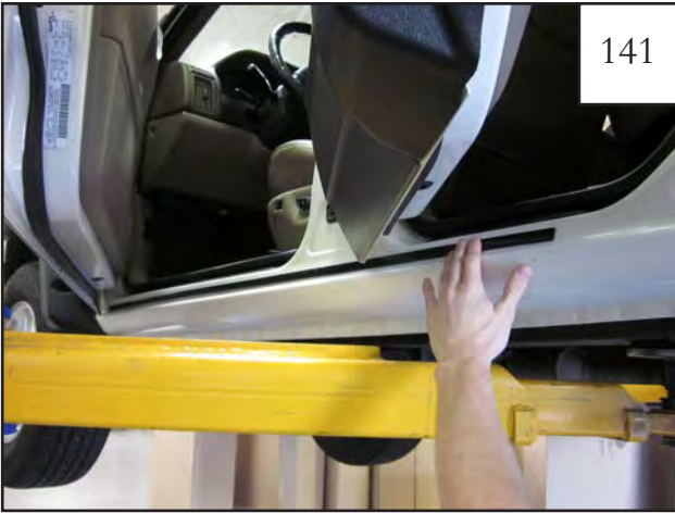
Remove tape liner from molding (GP1-0020) and starting at front hole, install molding along rocker area to cover holes in sheet metal.
