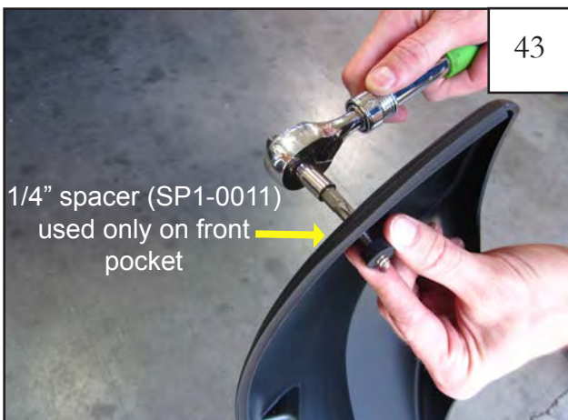
Install a Torx screw (SW1-0045) through FRONT pocket hole of flare and secure with rubber spacer ( SP1-0011 ) using supplied #45 Torx bit (SW1-0052). The torx bit fits into a 5/16" socket. Use with a 3-6" extension for drill or air ratchet. Drive screw into spacer until tight.
