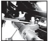
Step 3. Drill out the hole on the knuckle using a 13/16" drill bit. Carefully check the alignment when drilling to ensure a straight hole.
