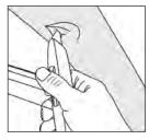
Use a Utility knife to cut a hole in the sport bar cover over the location of the hole. Repeat on opposite side of vehicle.
