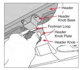
SECURE HEADER TO WINDSHIELD With the Bimini Centered on the vehicle, place the tabs on the Header Knob Bases above the footman loops in the windshield frame. Place a Header Knob
