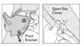
FOR VEHICLES WITH FACTORY SOFTTOP PIVOT BRACKET: PREPARE TO INSTALL WEB STRAP WITH GROMMET
