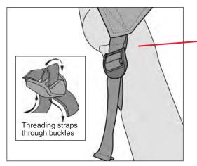
THREAD THE WEB STRAP THROUGH THE REAR BUCKLE Thread the Web Strap through the buckle sewn to the Bimini and pull it
