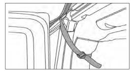
SECURE B-PILLAR STRAPS Wrap the strap around the B-Pillar between the front and rear door.
