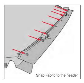
**Step One: for ALL '07- Current JK** SNAP BIMINI TO THE HEADER With the windshield header removed from vehicle, slide the pocket sewn along the front of the Bimini Top/Bimini Top Plus over the edge of the header and snap it to the eight snaps on both sides, as shown.
