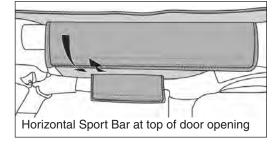
SECURE SIDE FLAPS Wrap the flap above the door opening around the horizontal sport bar and then fasten the hook and loop closure. Repeat on both sides of the vehicle.
