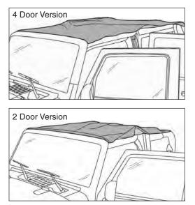
**Step Two A: for ALL '07- Current JK** DRAPE BIMINI OVER VEHICLE Drape the Bimini over the vehicle, and center it on the vehicle. Please see next page for continuation of step two.
