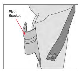
Soft Top Pivot Brackets, you may either use the M6 x 20mm bolt or re-install the factory bolt removed from the bracket in the previous step. The bolt goes through new hole in the sport bar cover.
