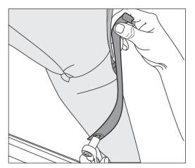
INSTALL WEB STRAP W/GROMMET Place the grommet in the web strap over the hole in the sport bar cover and secure the M6x20 Bolt. Repeat on opposite side of vehicle. For vehicles with Factory
