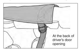
SECURE REAR CORNER STRAPS Locate the buckle straps sewn to the rear corner of the Bimini. Wrap the strap under the Bimini and around the sport bars. Thread the end of the strap through the buckle and pull it tight. Repeat on opposite side of vehicle.
