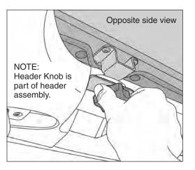
Plate under a footman loop. Install a Header Knob through the plate and footman loop and then thread it into the Header Knob Base. Repeat this process on the opposite side of the vehicle.
