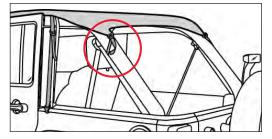
FOR VEHICLES WITHOUT SOFTTOP PIVOT BRACKET: PREPARE TO INSTALL WEB STRAP W/GROMMET Feel through the Sport Bar Cover and locate the bottom hole in the sport bar.
