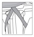
Thread the strap through the buckle and pull it tight. Repeat this on opposite side of vehicle.
