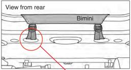
INSTALL SHORT TENSION STRAPS Drape the Bimini over the speaker pod. Thread a short tension strap through the
