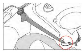
INSTALL LONG TENSION STRAP Thread a long tension strap thorough the buckle on the side of the Bimini.
