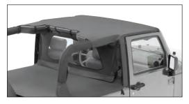
**Important:** For a smooth fit and ease of installation, this top should be installed at temperatures above 72 degrees. Below this temperature, the fabric may contract an inch or more making it difficult to install. We highly recommend taking the top out of the package and letting it sit inside a warm place or direct sun light for 1-2 hours before you install the top. When warm, this top will install quickly.
