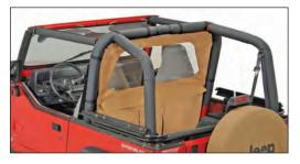
**Important:** For a smooth fit and ease of installation, this product should be installed at temperatures above 72 degrees. Below this temperature, the fabric may contract an inch or more making it difficult to install. We highly recommend taking the product out of the package and letting it sit inside a warm place or direct sun light for 1-2 hours before you install the top. When warm, this product will install quickly.
