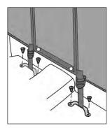
Use the holes in the Footman Loops as guides to mark, center punch and drill four 1/8 " holes. Seal the edges of the holes with Silicone Sealer. Install the Footman
