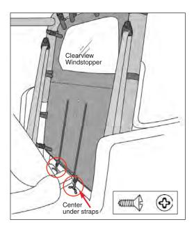
Loops using the four screws from the Footman Loop Kit. We suggest you do not remove footman loops once they are installed, but if you do, be sure to seal all holes with silicone sealer.
