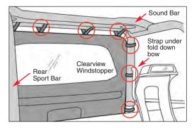
SECURE ALL CENTER/TOP STRAPS Orient the Clearview Windstopper with the window toward the top and with the vinyl side facing to rear of vehicle.
