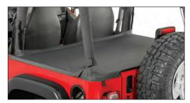
Important: For a smooth fit and ease of installation, this product should be installed at temperatures above 72 degrees. Below this temperature, the fabric may contract an inch or more making it difficult to install.
