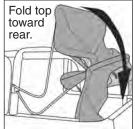
Raise front of the deck and collapse the rear bows, tucking the 2 plastic strips above the door openings and the "stay pad" on the rear bow inside of the bows, as seen in illustration above left.
