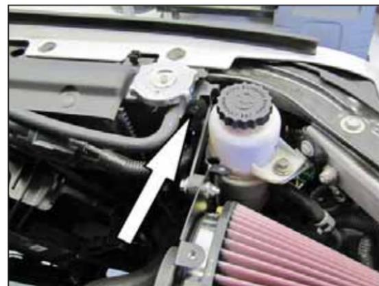
19. Install the heat shield bracket assembly onto the heat shield and radiator mount as shown. Secure the bracket with the factory bolt from step number 9 and the hardware provided.
