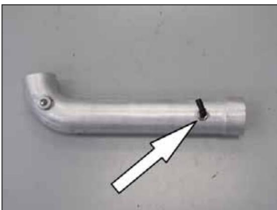
25. Install the 90°, ½" vent fitting into the K&N® intake tube as shown.
