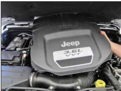
2. Lift up and remove the engine cover.
