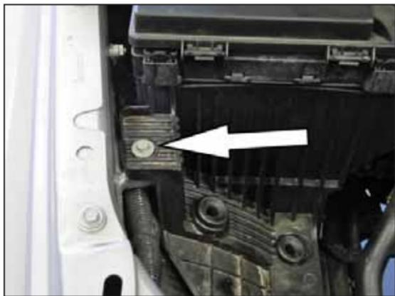
9. Remove the bolt show that secures the air box mount bracket to the inner fender.
