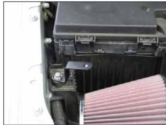
21. Install the provided bracket (083163) onto the rubber mounted stud using the provided hardware
