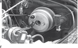
to installation. Take care that the rear plug insert of the Master Cylinder does not fall out.
