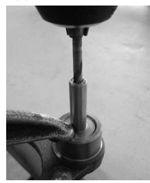
O Remove the Drill Guide and enlarge the hole using a 9/32" drill bit.
