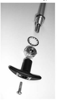
Insert the threaded end of the Actuator Cable (C) through the mounting hole from inside the engine compartment.
