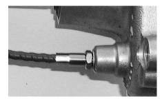
Reapply original grease to coil spring, splined collar and engagement fork and then reassemble as pictured below. Hint: Make sure splines on collar are well lubricated.
