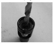
O Locate and remove the brass bushing and flat washer from the plastic plunger housing.
