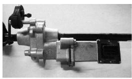
• Remove the three M10 bolts that secure the electric motor housing to the main gear housing. Separate the motor housing from the gear housing as pictured below.
