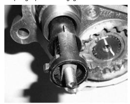
Pull the threaded end of the cable to remove any slack and thread one of the 1/4" Hex Nuts (C4) that was originally installed on the actuator cable back onto the stud. Tighten nut by hand.
