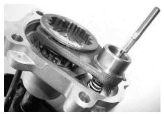
O Insert the supplied small rectangular Alignment Tab (A) into plunger mechanism directly over the drilled hole.
