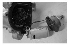
Using a wire cutter, cut the wires close to the electric motor and gearbox so that the remaining wires from the motor housing are long enough to work with. Discard electric motor and gearbox as they will not be used during reassembly.
