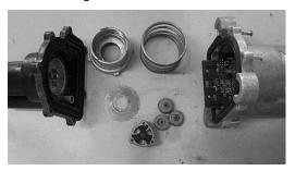
• Remove and discard all of the parts between the plunger housing and electric motor housing. These parts will not be reused.
