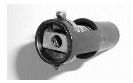
O Slide the plunger mechanism onto the Actuator Cable Stud (C5) and press fully into the plunger pocket in engagement fork.
