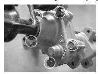
O Separate the main gear housing and retain the gasket seal for reassembly.
