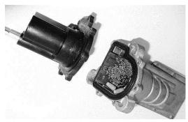
• Mate the motor housing to the main gear housing.
