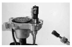
O Place the original gasket seal on the mounting flange of one of the main gear housing halves.
