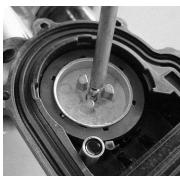
O Using a 1/8" punch, carefully drive the worm shaft through the worm shaft coupler.
