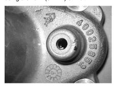
O Using a 5/16" -24 thread tap, cut threads in the enlarged hole.
