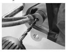
O Remove the Drill Guide and enlarge the hole using a size I (0.272") drill bit.
