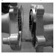
Remove the coil spring, engagement fork and splined collar from the main gear housing.
