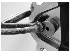
O Using a 3/16" drill bit, insert the drill into the guide and drill a pilot hole through the housing.
