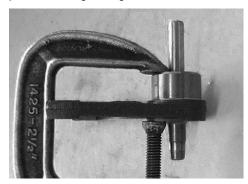
O Using a 3/16" drill bit, insert the drill into the guide and drill a pilot hole through the engagement fork.
