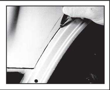
Step 8. Trace a horizontal line from the previous line in step 7 toward the inside of the fender well at the top of the third factory mounting hole. Repeat for opposite side.
