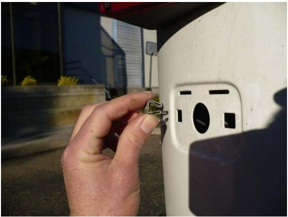
4) With both inserts removed, note the "UP" orientation of the 5103 JK license plate delete panel and install into the tub. The panel should snap into position and secure itself to the tub. Completed part installation should appear as shown below.
