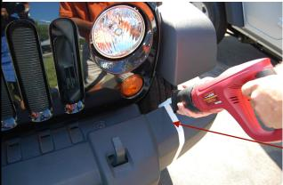
2) Using a Reciprocating Saw cut along the INSIDE edge of the tape line where you measured at the 3 1/2" Mark
