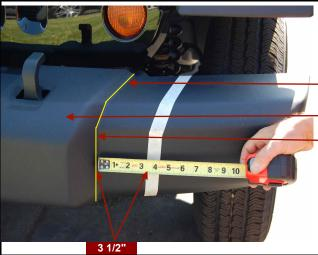
1) Measure 3 1/2" from the Bumper Pad toward the outside of the bumper both on the top of the bumper and the front of the bumper and mark with tape
