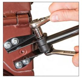
**Step Four: Adjust Arm Tension** Once the mirror head is installed, snug the bolt and nut that secure the mirror arm to the mounting bracket. Adjust the tension to achieve the desired setting of the mirror. Over tightening will not allow the mirror to be adjusted properly.
