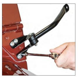
**Step Two: Install Mirror Arm** Install the new mirror arm using the supplied hardware. Each of the four mounting holes should get a flat washer, a lock washer, and a bolt, in that order. Snug all four bolts using a 10mm wrench or socket. Do not over tighten.
