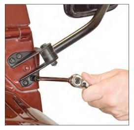
**Step One: Old Mirror Removal** Put on safety glasses. Remove old mirror by removing the (4) T30 torx fasteners that attach it to the windshield frame. Locate the appropriate Mirror for the first side you are installing. Mirrors are stickered "R" for right (passenger side) and "L" for left (driver side).
