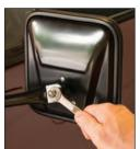
Snug the acorn nut and the standard nut together using a 12mm wrench and a 12mm socket. Do no over tighten.
