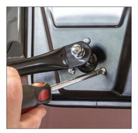
**Step Five: Adjust Head Tension Screws** Adjust the 3 tension screws on the backside of the mirror in order to achieve proper adjustment. Once again, do not over tighten or you will not be able to properly adjust the mirror head. Periodic adjustment may be necessary to retain the correct tension. Finally, repeat all steps for mirror installation on the opposite side of vehicle.
