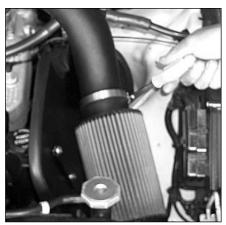
16. Install the K&N Filtercharger onto the K&N intake tube as shown.
