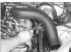
14. Install the provided silicone hose onto the crankcase vent, then install the other end onto the K&N intake tube.
