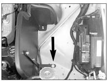
10. Using the provided hardware, secure the "L" bracket to the inner fender as shown.
