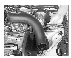
15. Install the provided silicone hose onto the EVAP canister vent line then secure the other end onto the K&N intake tube.
