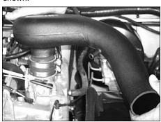
13. Install the K&N intake tube onto the throttle body and tighten the hose clamp.
