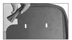
7. Install the trim seal onto the heat shield. Trim excess if needed.
