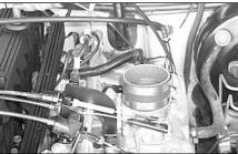
12. Install the silicone hose and the hose clamps onto the throttle body as shown.
