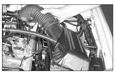
4. Loosen the hose clamp at the throttle body and unclamp the airbox lid then remove the upper intake assembly as shown.
