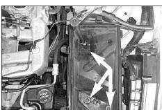
5. Loosen and remove the two bolts and one hex nut that secure the lower air cleaner assembly.
