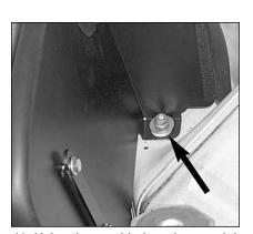
11. Using the provided washers and the hex nut removed in step 5, secure the heat shield assembly to the existing stud as shown.
