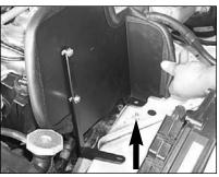
9. Install the heat shield assembly into the vehicle lining up the factory stud with the tab on the heat shield.
