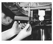
21 Lower the axle onto the spring, being sure to center the spring center bolt in the hole on the axle spring pad. Next, install the U-bolt skid plates.
