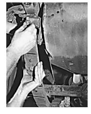
18 With the rear axle supported securely on jackstands, remove the upper shackle mounts from the frame. Be careful not to break off the bolts in the frame.
