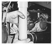
15 Install the Old Man Emu shocks. On some vehicles, it may not be necessary to use the supplied shock mounts. IMPOR-TANT: Remember to check the brake line for appropriate length when the suspension is at full drop and compression with wheels turned. You do not want to overextend and damage or separate the brake line due to the increased suspension travel.On some vehicles, it may not be necessary to use supplied shock mounts.Optional: Install Rock Equipment sway bar disconnects-male end up.
