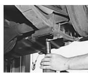
17 Set the rear of the vehicle on jack stands and remove the U-bolt spring plates and spring.
