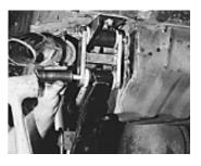
19 Install the new Rock Equipment shackle hanger using the existing holes in the frame. Install bushings in the spring and hanger, then install using the greasable bolts and sleeves.
