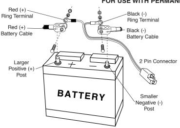
For batteries installed in vehicles or other equipment we have provided a lead set with ring terminals. Since many installed batteries are in space-restricted locations or compartments, these ring terminals (see illustration to left) have been designed to provide a safe and convenient connection. Follow these steps for connection and operation:
