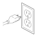
Connect the Battery Extender to a grounded 120 Volt AC power receptacle (left) that is wired in compliance with local electrical code. A grounded receptacle will receive a plug with a round ground pin and two blade terminals.
