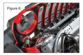
gently pop the grille from its lower retainer clips. Once the grille is removed and/or tilted forward, locate the chrome trim rings around the Headlights. Using a T15 Torx screw driver, remove the factory headlight trim ring on each headlight (Fig 8). Place the removed screws (4 per light) in a safe place as they will
