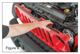
Helpful Hint: If you are installing the Euro-Guards by yourself or are also installing turn signal Euro-Guards, you may want to completely remove the grille from the front of the vehicle.
