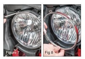
be re-used to install the Headlight Euro-Guard. With the chrome trim ring removed, place the front Euro-Guard trim ring (each will fit either side) over the headlamp lining up the tabs as shown below (Fig 9). When installed, the Euro-Guard bars will be vertical and each tab will align in a slot on headlight housing.
