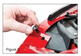
Depending on your model year, pry up or unscrew the plastic fasteners (6 total) using a small screw driver. Early vehicles may feature phillips head screws, but most vehicles have a pry-up rivet as shown (Fig 2). First remove the center, then remove the body of each plastic retainer (Fig 3). Set rivets & screws aside in a safe place for re-installing the grille.
