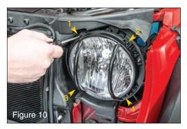
At this point the Front Headlight Euro-Guards are installed. If you plan to install TACTIK® Turn Signal Euro-Guards we recommend installing them at this point as you will have best access to the mounting points.
