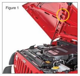
Put on safety glasses. Open the hood of your Jeep<sup>®</sup>. Put the prop rod into the correct slot to hold hood open (Fig 1).
