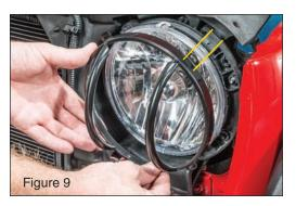
Repeat this sequence for the other side. With the Torx head screws you removed in step 3, partially reinstall each screw into the 3 alignment tabs (Fig 10). Do not tighten yet. Starting from left to right, tighten each screw an even amount to "pull" the Euro-Guard tight onto the headlight (Fig 12). Repeat for the other headlight.
