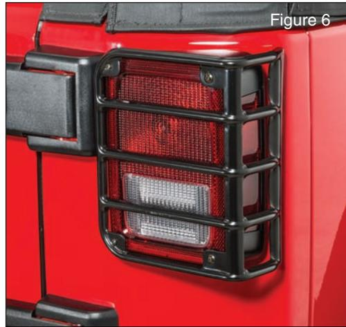
**Step Three: Tighten Mounting Screws**
