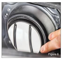
From under the vehicle, place the driver's side Euro-Guard into the Fog lamp opening on the back side of the bumper. The Bars on the Euro-Guard should be in the vertical position (Fig 5).
