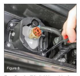
Euro-Guard will be held in position between the light housing and the bumper itself. With driver side now complete, please repeat all steps for the passenger side Fog Light Euro-Guard.
