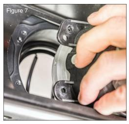
A helper can be handy to hold the Euro-Guard in place (Fig 7), Carefully re-install the Fog Lamp housing into the bumper using the original Phillips head screws. Snug the screws (Fig 8) and the
