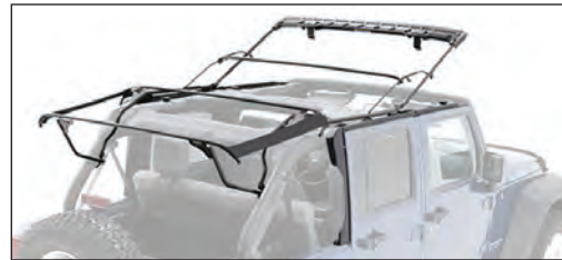
Existing soft top hardware required to install this top. Does yours match?
