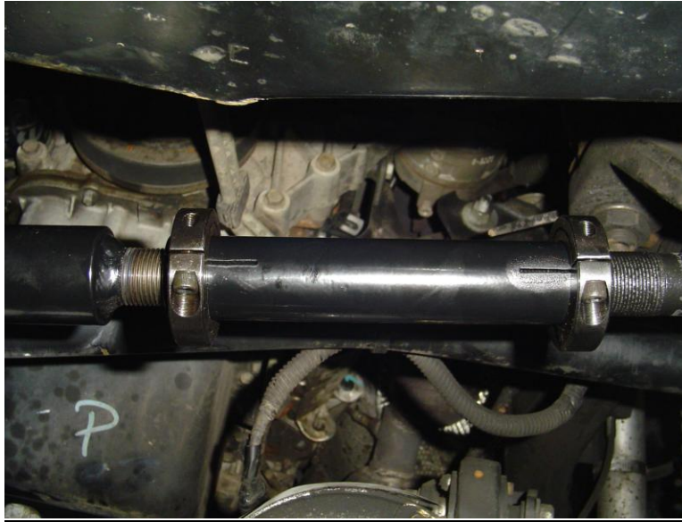
Quick adjuster with shaft collars installed
