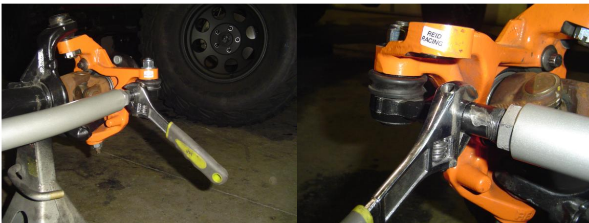
Tighten drivers side first with wheels straight
