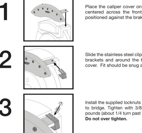
Place the caliper cover on the brake caliper. Cover should be centered across the front. Caliper cover bridges should be positioned against the brake caliper bracket.
