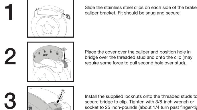
Install the supplied locknuts onto the threaded studs to secure bridge to clip. Tighten with 3/8-inch wrench or socket to 25 inch-pounds (about 1/4 turn past finger-tight). Do not over tighten.
