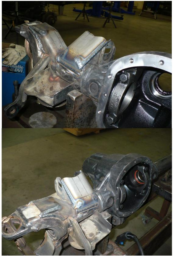
6) After welding, clean off any weld burrs and paint to the desired color to prevent corrosion.
