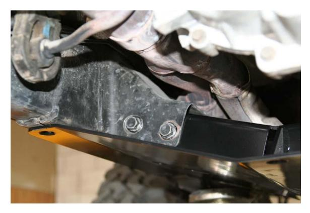
7. At this time, mark and drill the holes for the countersunk bolts. There are 4 total for the transmission skid.
