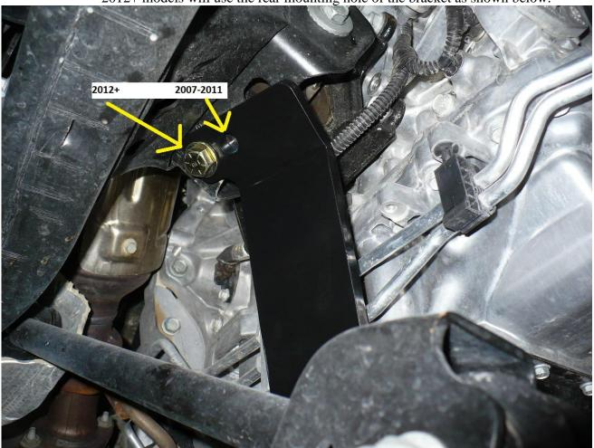
18. Install the engine skid plate at this time. All hardware should still be loose at this point. Install the skid plate by bolting it to the motor mount brackets using the supplied 3/8" hardware in the kit. Again use a lock
