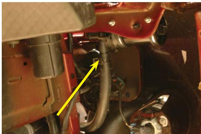
139. Cut 1-1/2" off the end of one of the supplied 4" x 36" x 90° elbow hoses.
