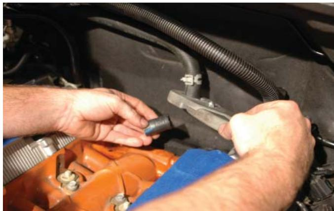
57. Install the provided 5/8" 90° elbow on the end of the hose you just cut. Secure the elbow on the hose so that the open end points toward the driver side fender and the handles of the hose clamp point toward the passenger side fender.
