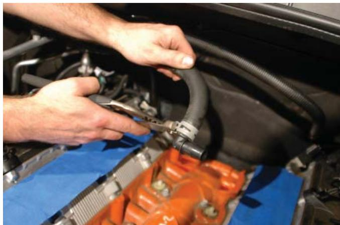
58. Attach the supplied 5/8" x 48" hose to the driver side barb installed on the water pump using a supplied spring clamp.
