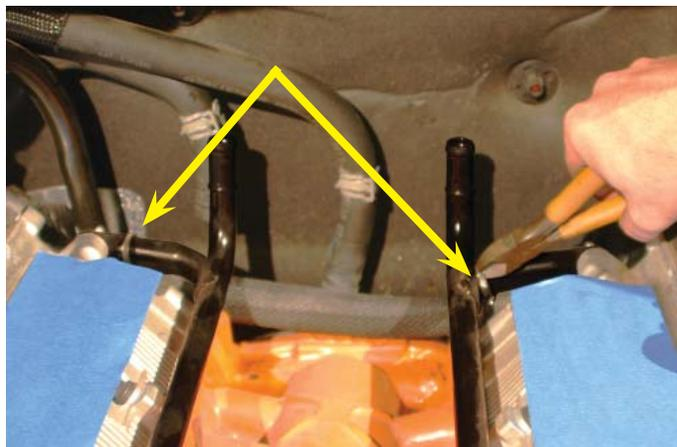
38. Use a 10mm wrench to remove the studs holding the two heater hard lines to the back of the heads.
