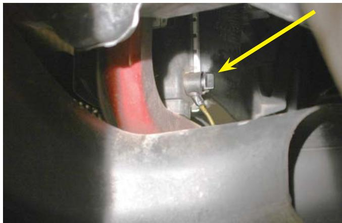
6. Remove the radiator cap to facilitate draining. Upon drainage completion, replace the cap loosely and tighten up the drain valve.
