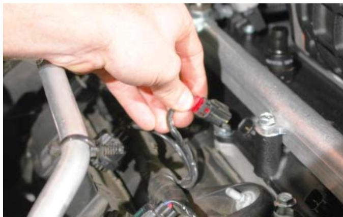
104. The IAT extension harness should be exiting below the supercharger intake manifold assembly on the passenger side of the engine. Connect the extension to the existing IAT plug and tuck the wires under the throttle body upon completion.
