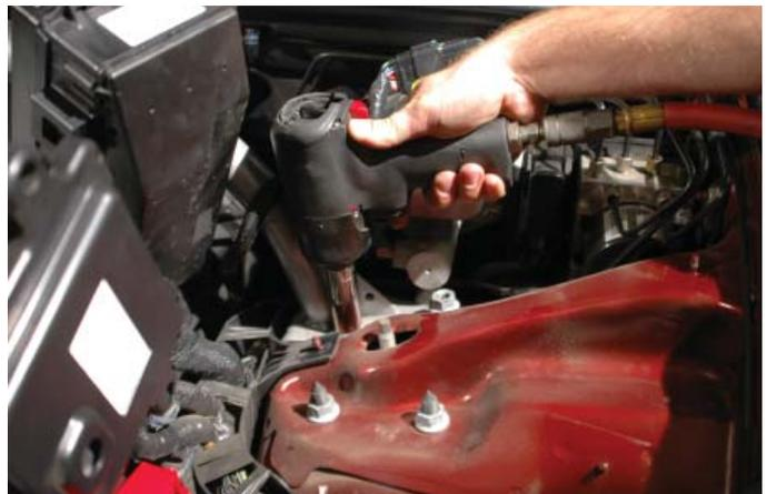
15. Pull up on the strut tower brace to pull it off the studs. On the driver side, the mounting flange will hit the bottom of the brake cylinder. Pull the brace completely off the passenger side, and angle the brace to the rear to gain clearance to further pull the strut tower brace from the vehicle. Set aside for later use.
