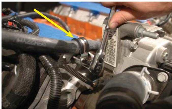
52. Install the supplied  $\frac{3}{4}$ " -5/8" coupling (hose mender) in the supplied  $\frac{3}{4}$ " x 7" section of hose. Secure in place with a supplied spring clamp.
