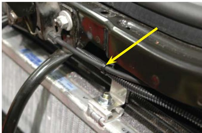
153. Connect the intercooler relay harness plug to the receptical on the intercooler pump.
