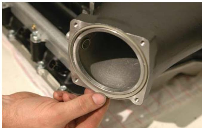
88. Install the throttle body on the new supercharger intake with the motor pointing down. Use the stock bolts removed from the OEM manifold and torque to 106" lbs. Verify your torque wrench settings.
