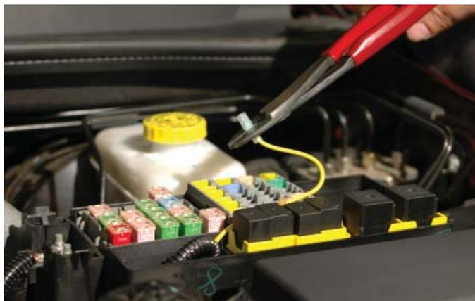
160. Route this wire over to the fuse tap just installed and plug the spade end onto the fuse tap. Bend the wire over toward the center of the box and close the cover.
