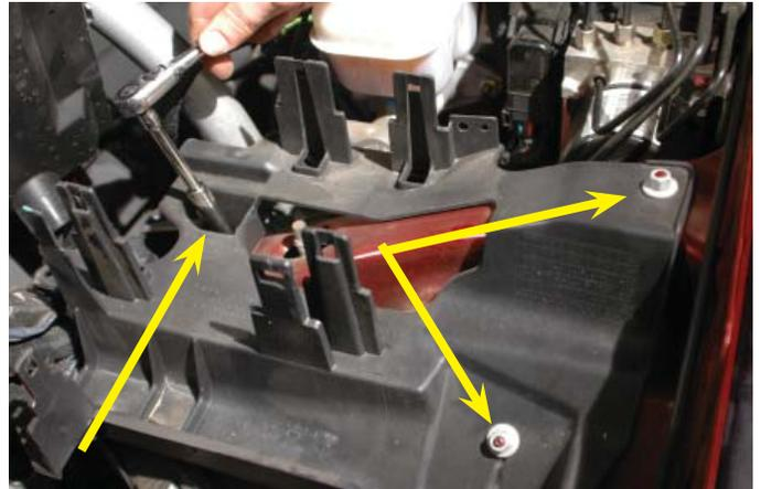
14. You now have access to the driver side bolts holding the strut tower brace in place. Use an 18mm wrench to remove the nuts securing the strut tower brace in position (two each side). We used an impact wrench but this is not necessary.
