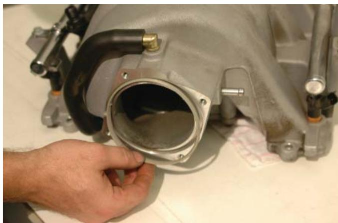
87. Install the throttle body gasket on the new supercharger inlet. If you have trouble with the gasket staying in place, more clearance can be achieved by cutting the small tabs off the gasket.
