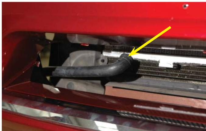
136. Continue to route the hose around the radiator support frame, in and over the lower radiator hose and up into the engine compartment on the passenger side over the coil packs back toward the rear of the vehicle.
