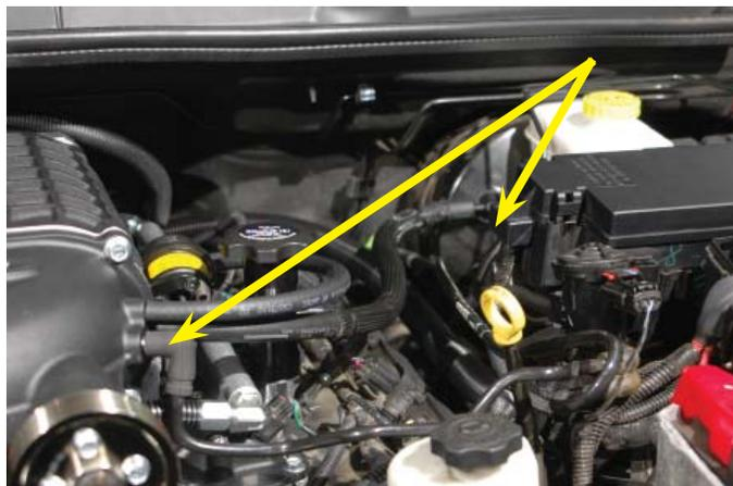
110. Install the fuel line on the new fuel manifold barb at the rear-passenger side fuel rail.
