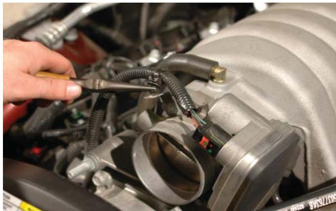
21. Disconnect the ETC from the throttle body. To achieve release, first press the red lock clip up to release the lock, then squeeze below the lock clip and pull the ETC away from the throttle body.
