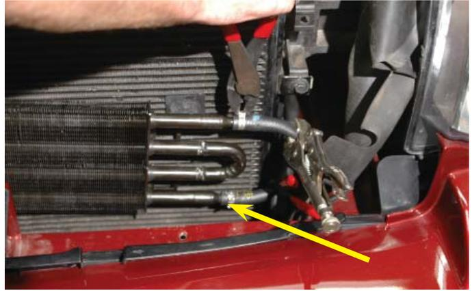
69. The existing power steering cooler plastic mounting tabs will have to be removed. We found the easiest solution was to use a saw blade to cut the tabs off of the mounting plate.
