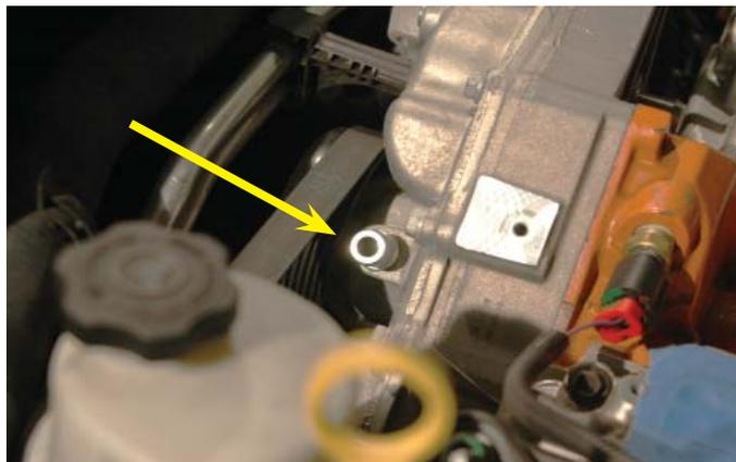
49. Remove the stock center-most heater hose from the firewall hose barb on the passenger side of the engine compartment.
