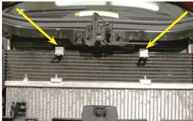
73. Slide the intercooler heat exchanger up and secure to the located mounting brackets using the provided nuts.
