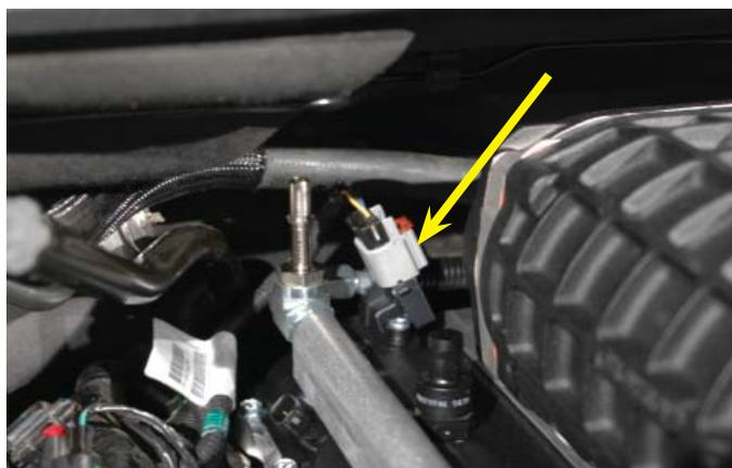
103. Connect the eight fuel injector plugs. Ensure that they clip securely in place.
