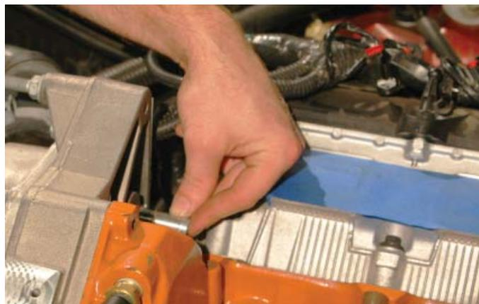
48. Use your fingers to press the other prepared barb into the driver side hole of the water pump that was vacated by the removal of the driver side hard line heater pipe that ran under the OEM intake manifold.
