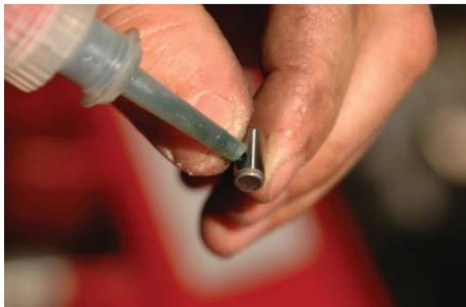
194. Insert the pins in the prepared holes and tap in using a punch. Make sure the pins are all the way in, the crank pulley bolt should not be able to touch the surface of the pin.
