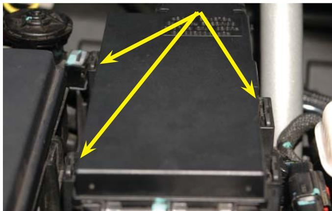
12. There is a wiring harness that has two clip locations that tie the harness to the fuse center mounting bracket. Pry these harness clips off of the fuse center mounting bracket.
