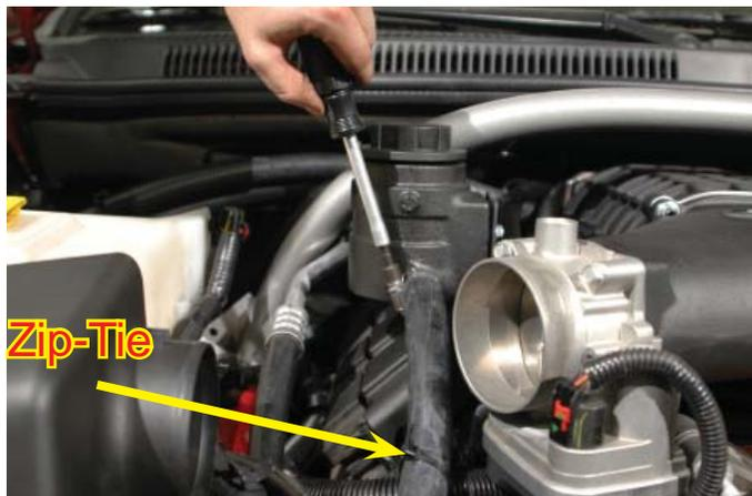
146. Route the hose from the passenger side barb of the supercharger intercooler to the rear hose barb of the intercooler reservoir, cut to fit and secure in place using a provided worm gear clamp.
