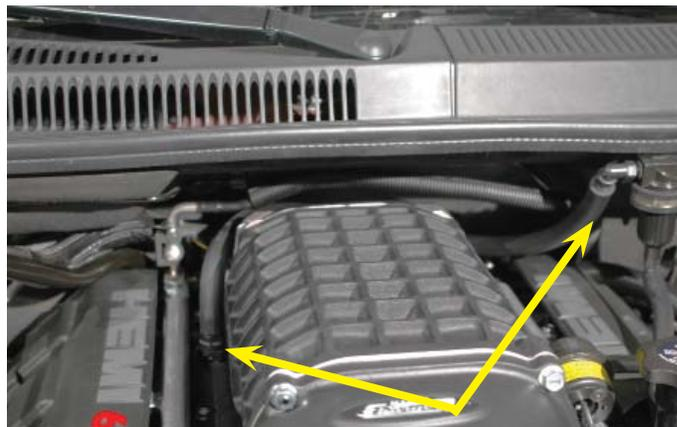
117. Install a 42" piece of the supplied 1/2" hose between the passenger side barb on the supercharger inlet and the driver side barb of the oil separator valve.
