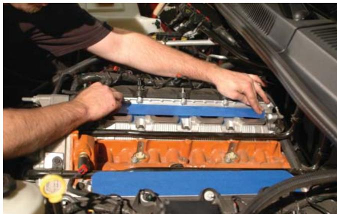
34. Remove the two heater hose clamps from the hard line barb at the rear of the valley by the firewall, they run over the valley to the water pump.
