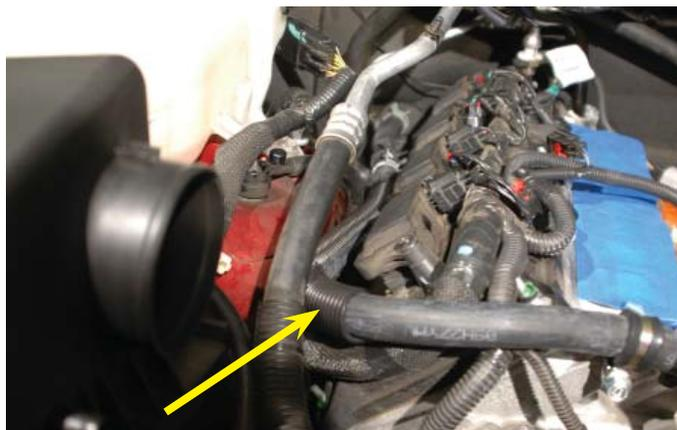
56. Cut about 1-1/2" from the end of the other heater hose at the firewall that used to run to the driver side hard line running under the OEM intake manifold.
