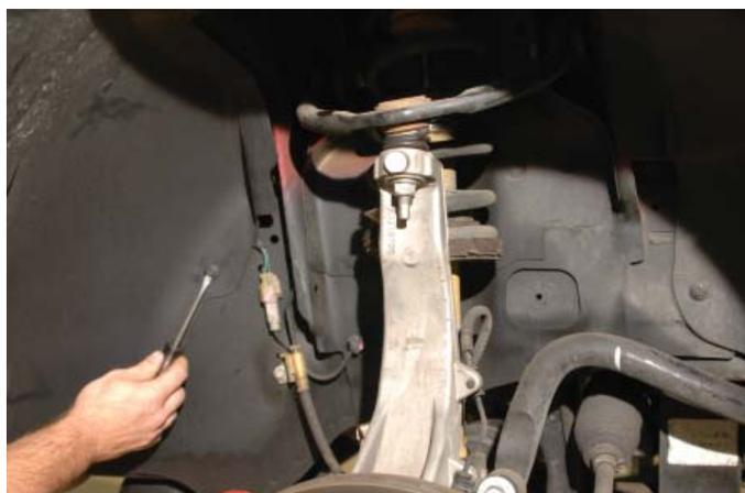
127. There are five plastic 'pop' rivets. Use an awl or tiny screwdriver to push in on the center post of the rivets to release the lock, the rivets can then be pulled free.
