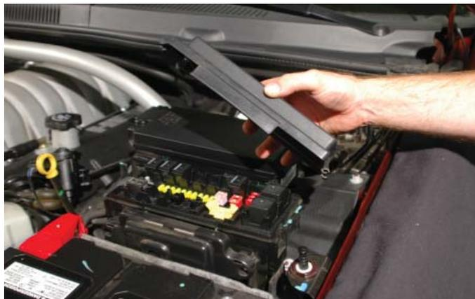
9. With the cover removed, use a small screwdriver to release the three hold down clips. The forward fuse center should now be free to pull up.
