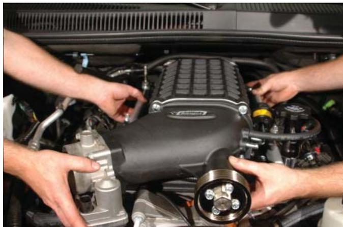
101. Torque the supercharger mounting bolts to 106" lbs using a center-out, criss-cross pattern. Verify your torque wrench settings.
