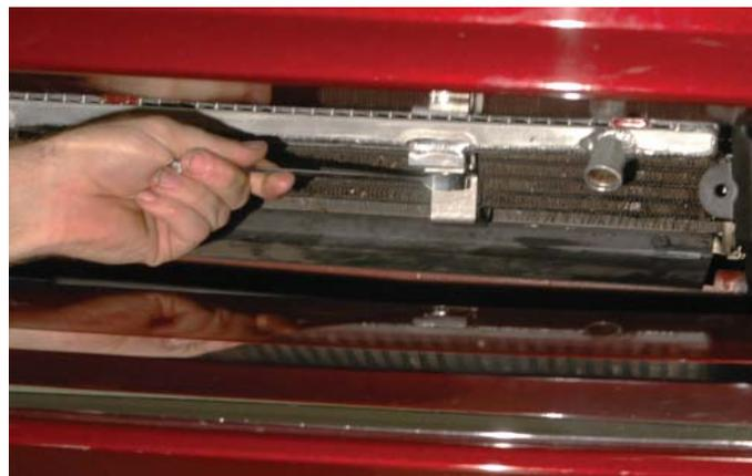
76. Flip the power steering cooler over so that the mounting tabs that were originally on the rear are now facing forward. Slide the provided crimp clamps onto the power steering hoses that you pinched off earlier and press the hoses back onto the power steering cooler hose barbs. Securely crimp the hoses onto the barbs using crimp pliers or dykes, be careful to not cut the clamps.
