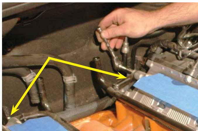
39. The driver side heater hard line has two additional mounting bolts. Use a 10mm wrench to remove the center mounting bolt from the middle of the valley.
