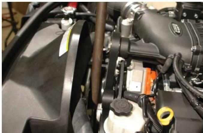
183. Replace the AC mounting bracket back on the post in front of the engine.
