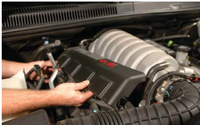
17. Disconnect the IAT sensor plug at the intake air tube.
