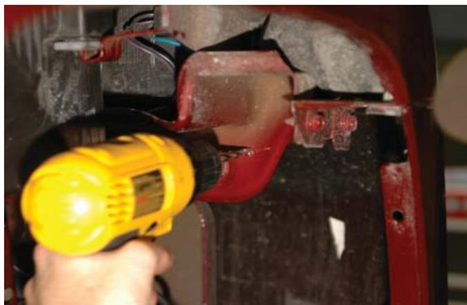
131. The pump will mount to the forward side of the hole you just drilled and the existing hole toward the center in this configuration. **Note that the spacers will be against the cross brace, the clamp comes next with the lobes pointing down and forward.**
