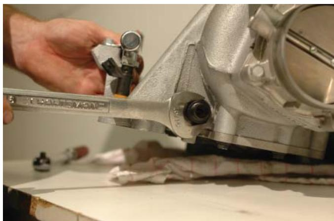
83. Install the PCV valve in the passenger side hole of the supercharger lid and tighten with 15/16" wrench.
