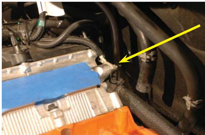
46. Place a generous bead of the supplied Green Loctite on the two supplied water pump hose barbs.
