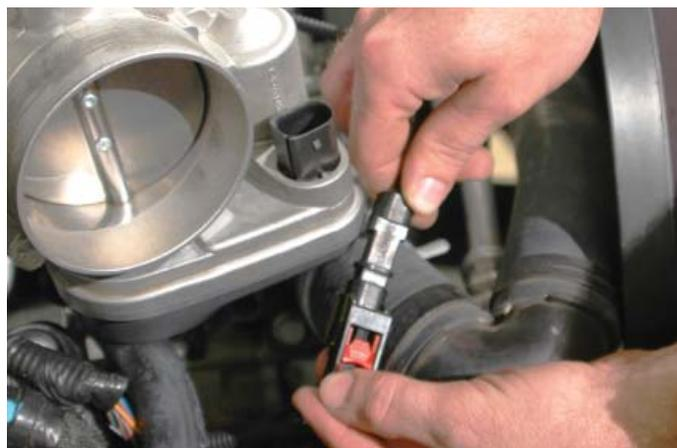
105. Plug in the throttle body connection.
