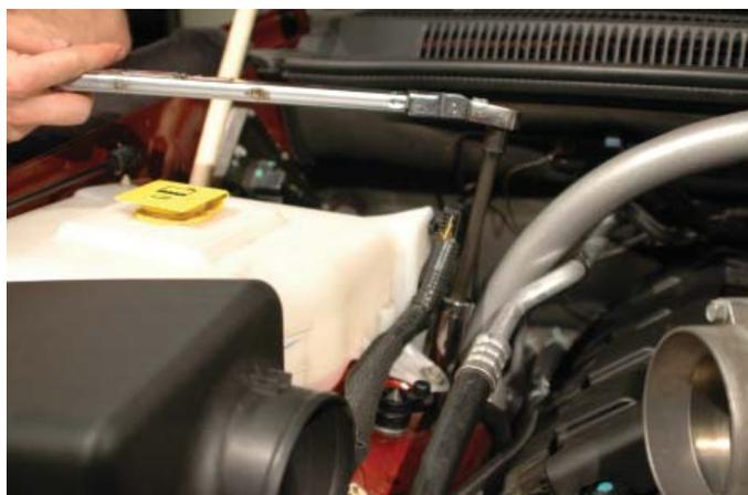
119. Install the fuse center mounting bracket using the original three nuts and tighten using a 10mm wrench.
