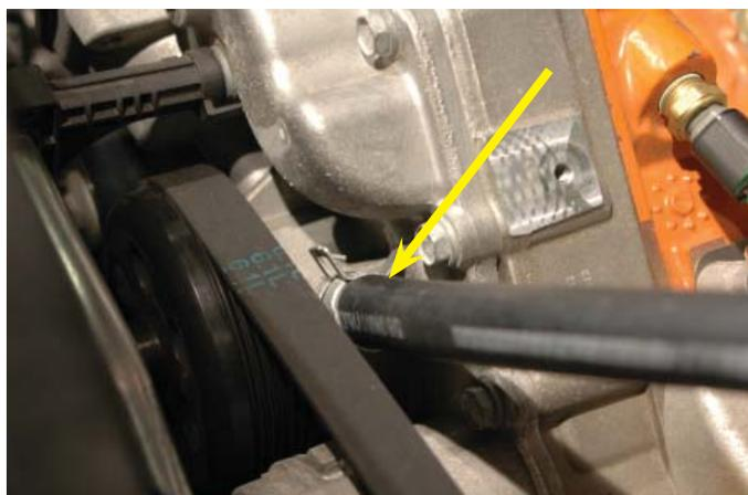
59. Use the bolt hole on the front of the driver side head, the supplied spacer, then Adel clamp and bolt to anchor the hose you just installed to the engine. The lobe of the Adel clamp should be pointing up and toward the front of the vehicle.
