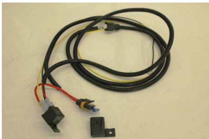
151. Pull the hood release cable down from under the upper cross brace adjacent to the windshield washer reservoir cap. Use the provided zip-tie to tie the fuse holder and relay close to the washer reservoir.
