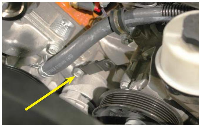
176. Attach the supplied idler bracket to the top water pump bolt location and the supercharger pulley support using the provided bolts. Torque to 20 ft lbs.
