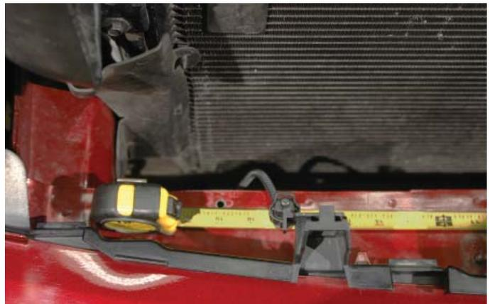
72. Slide the two carriage bolts into the slots of the intercooler heat exchanger and place the heat exchanger just in front of the air conditioning condenser on top of the bumper support. Use the location of the two bolts to locate where to place two of the prepared intercooler heat exchanger mounting brackets. Press the mounts into position on the air conditioning condenser top tank.
