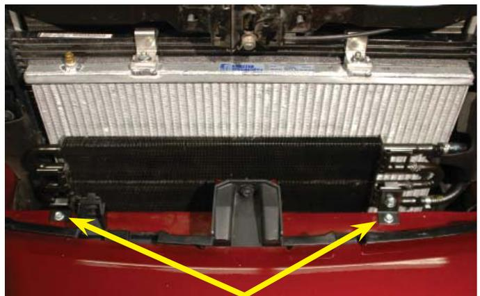
80. Re-attach the fascia braces on either side of the hood latch in their original location using the factory hardware and tighten securely.
