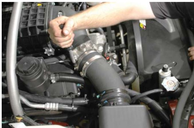
170. Near the front-center of the engine is a plastic mount anchoring the AC hard line to a stud. Pry this mount off the stud using a large flathead to get a little more room.
