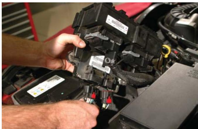
11. Again use a small screwdriver to release the locking clips of the rear fuse center located just forward of the brake reservoir. Pull the rear fuse center up off the mounting posts and push it over toward the engine with the forward fuse center.
