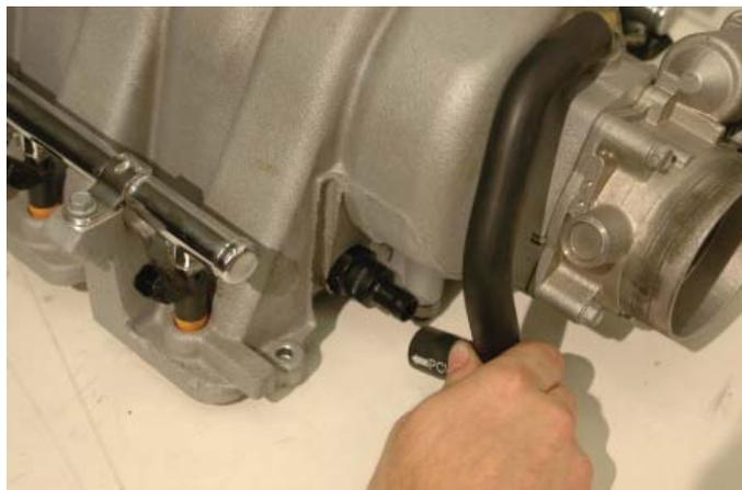
82. Use a 15/16" wrench, remove the PCV valve from the stock intake manifold.
