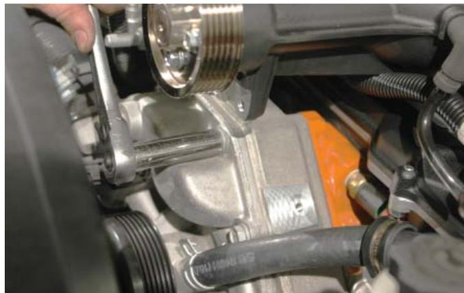
173. Loosen the tensioner assembly using a 15mm wrench. This does not need to be removed just loosened enough to remove the next bolt.
