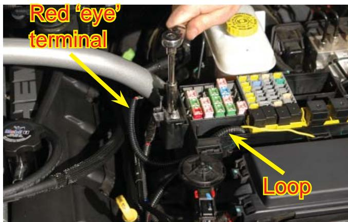
155. Replace the nut incorporating the "eye" on the end of the red wire of the relay harness.
