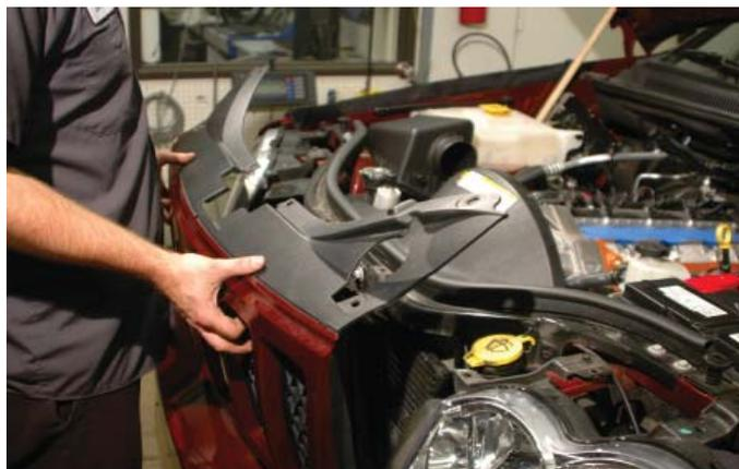
64. Cut strips of the supplied adhesive backed rubber and apply to the inside surfaces of the heat exchanger mounting brackets, on top of the strips applied, cut and add the ½” adhesive backed rubber as shown.
