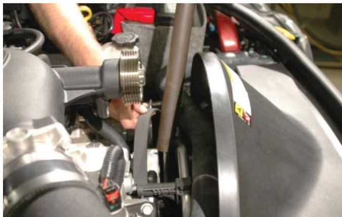
172. Remove the top water pump bolt using a 13mm wrench.
