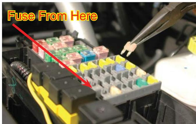
157. Add the fuse tap supplied to one leg of the 25A fuel pump fuse.
