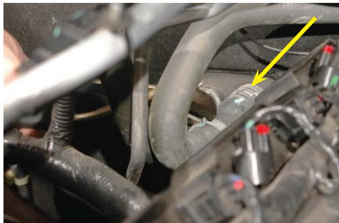
50. Cut 2-1/2" off the short end of the supplied 4" x 48" x 5/8" 90° elbow hose and attach the short end to the barb just installed on the passenger side of the water pump using a provided spring clamp.
