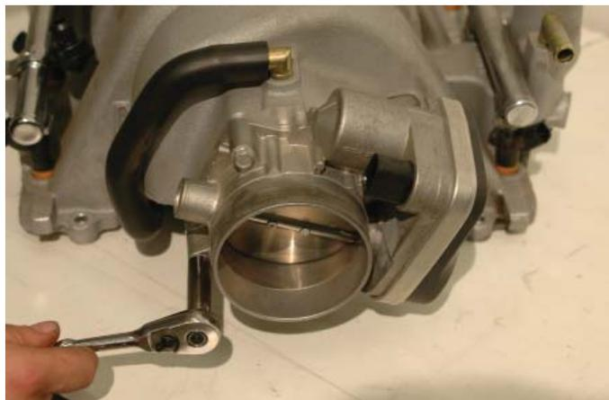
86. Remove the throttle body gasket from the OEM manifold.
