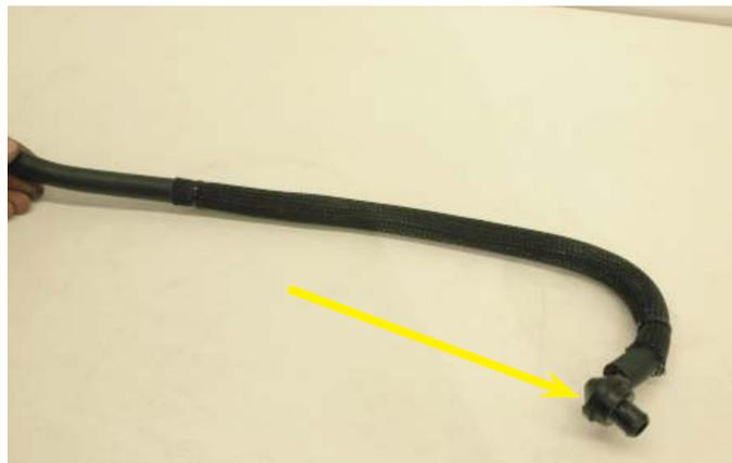
109. Connect the brake booster valve to the brake booster canister and route the hose forward to connect to the hose barb on the supercharger inlet as shown.
