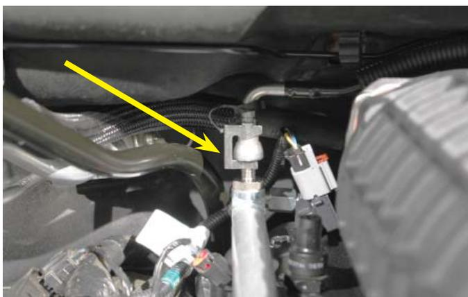
112. Extend the 'lobe' of the notch in the driver side coil pack cover approximately 1" further toward the rear of the cover and press in place over the coil packs in the original location. This modification is to create clearance with the oil separator drain hose to be installed next.
