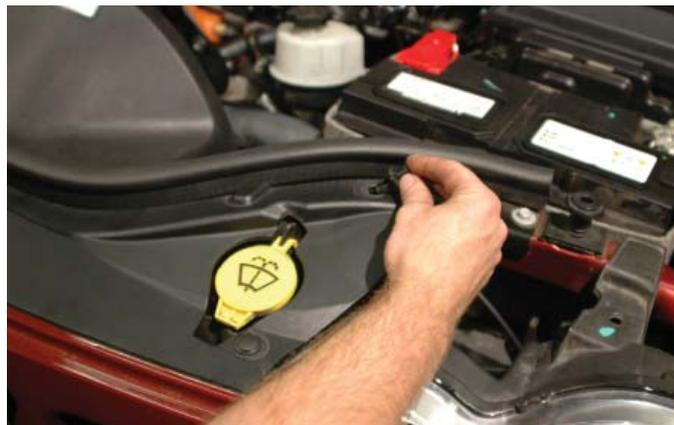
201. Find a place to loop the cable of the OBD port (a panel behind the port can be opened and the cable looped around the wire harness inside) and press the cover over the port.
