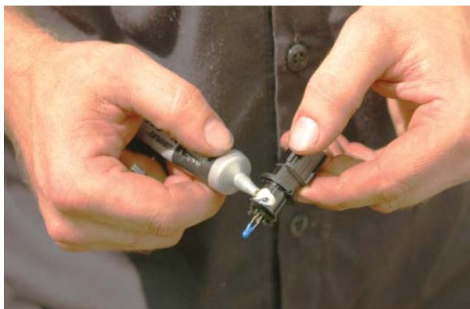
91. Flip the supercharger assembly upside down onto clean shop towels. Remove the bolt and mounting bracket over the IAT grommet temporarily. Press the IAT sensor into the grommet in the bottom of the supercharger assembly with the notch in the stop ring pointing toward the mounting bolt hole. Secure in place with the tongs of the mounting bracket and bolt.
