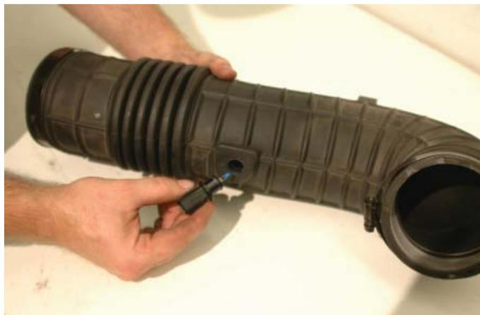
90. Lube the O-ring of the removed IAT sensor with the provided Lubriplate lubricant.
