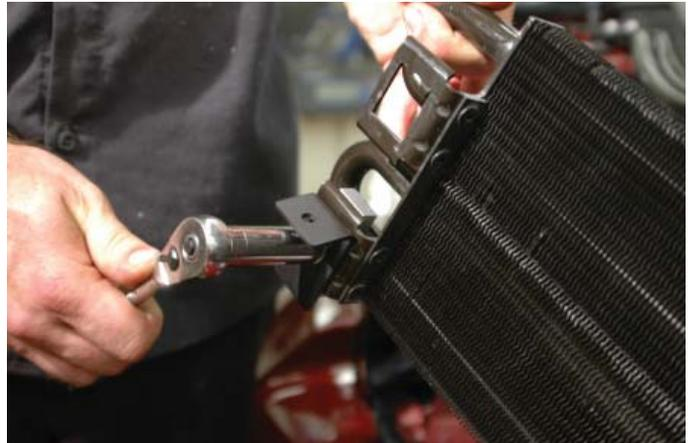
78. Attach the obtuse (greater than 90°) angle mounting bracket to the driver side lower mounting bracket using the supplied threaded plate with the angle being down leg pointing forward. Fingertighten the bolt to the backing plate at this time.
