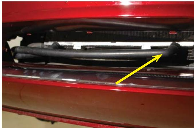
138. Cut the hose to fit and connect to the intercooler pump discharge barb using one of the provided spring clamps.
