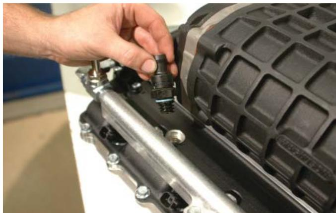
84. Remove the oil fill cap from the OEM manifold assembly and install on the new supercharger oil fill spout.
