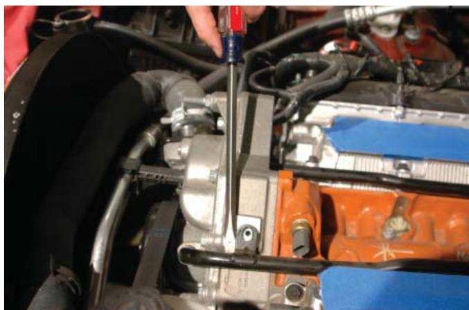
43. On the passenger side the heater hard line needs to be pulled toward the rear to remove it from the water pump. Use the large screwdriver with the head as a fulcrum to lever the hard line free from the water pump.
