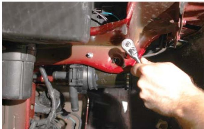
133. Roll the clamps forward and up after tightening and twist the pump to keep the discharge barb pointing down.
