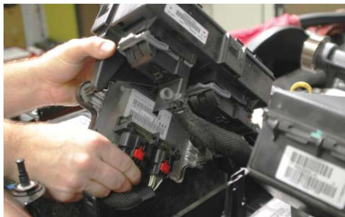
121. Install the forward fuse center onto the three fuse center mounting bracket posts. An audible click is heard when locked in place.
