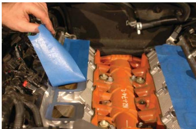
99. Wipe any tape residue or debris off using lacquer thinner or alcohol or some other suitable non-petroleum based solvent.
