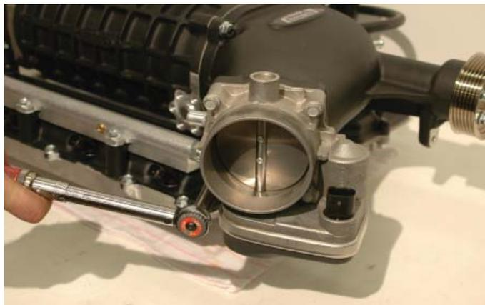
89. Remove the factory IAT sensor from the OEM air tube.
