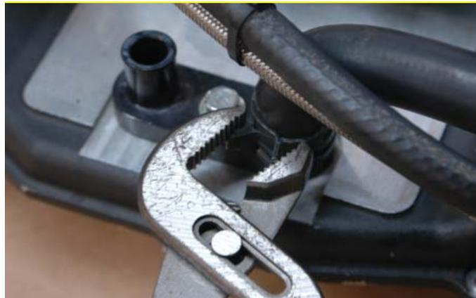
97. Connect the short end of the other modified 4" x 36" x 90° elbow hose to the driver side intercooler hose barb behind the supercharger using a provided spring clamp. This hose will also route toward the passenger side of the vehicle.
