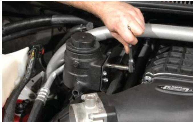
145. Route the hose from the intercooler pump inlet barb to the forward barb of the intercooler reservoir bottle. Tie the hose down to the existing harness below the throttle body using a supplied zip-tie, cut the hose to fit and secure to the reservoir bottle using a supplied worm gear clamp. **NOTE: It's important to use worm gear clamps on the reservoir bottle.**
