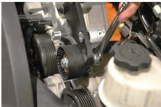
179. Install the second idler pulley using the supplied bolt. Use a 14mm wrench and torque the bolt to 40 ft lbs.
