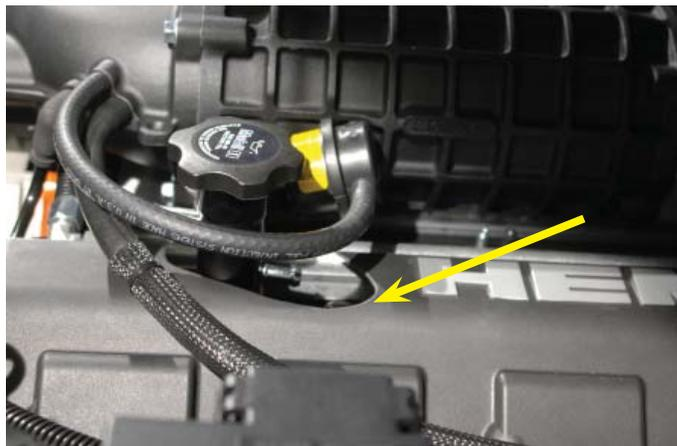
113. On the driver side below the windshield cross brace is an existing stud pointing down. Use the provided nut to attach the provided bracket to the stud and tighten with a 10mm wrench.
