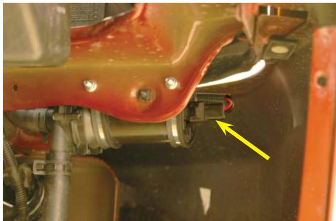
154. Tuck the yellow wire into the split loom covering the red wire from the relay. Route the two wires into the engine compartment over to the rear fuse center on the engine side. Tuck a loop of the harness up into the forward cavity of the fuse center, and pull the yellow wire out of the split loom at the peak of the loop. Remove the nut from the positive post of the fuse center.
