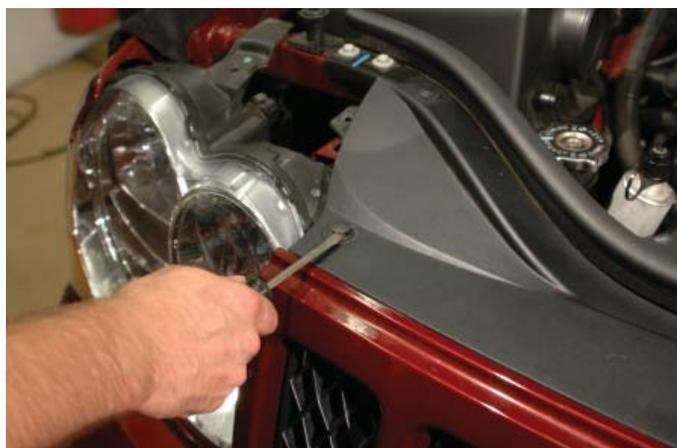
63. Pull forward and up to remove the fascia grille. Set aside in a safe location for later re-install.
