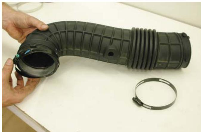
167. This is the air tube components, including the two clamps removed from the OEM unit.
