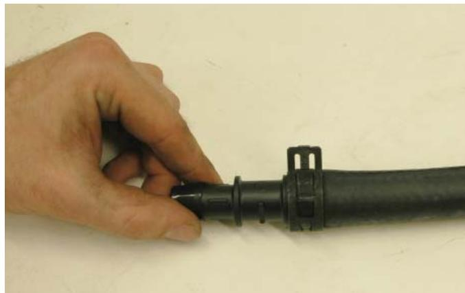
53. Use the stock clamp removed from the OEM heater hose removed earlier to attach the 7" piece of hose to the center-most heater barb at the firewall on the passenger side of the engine compartment.
