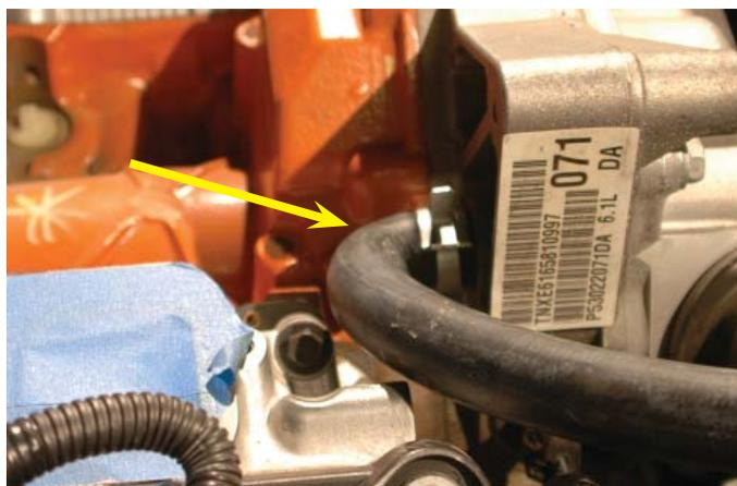
51. Route the hose toward the passenger side fender. Use the bolt hole at the front of the passenger side head near the water pump, add the supplied spacer, then the Adel clamp with the lobe up and pointed toward the rear of the vehicle, and the supplied bolt to anchor the heater hose as shown in this picture.
