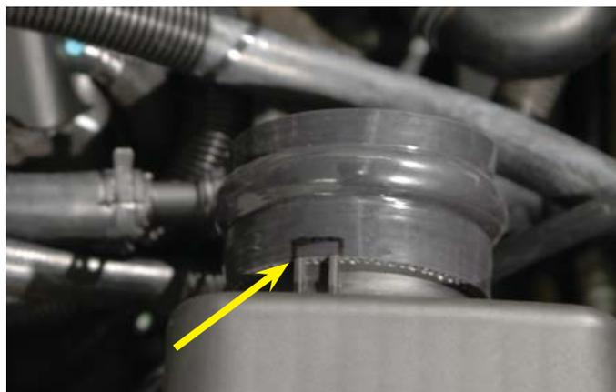
169. Install the notched hose in place on the air box. Slide the other hose completely onto the new air tube throttle body end. Press the air box end of the air tube into the receiving end of the hump hose...rotate the air tube to fit and slide the straight hose onto the throttle body. Tighten all clamps securely.
