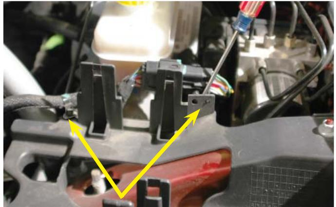
13. Use a 10mm wrench to remove the three nuts holding the fuse center mounting bracket to the strut tower/interior tire well studs.
