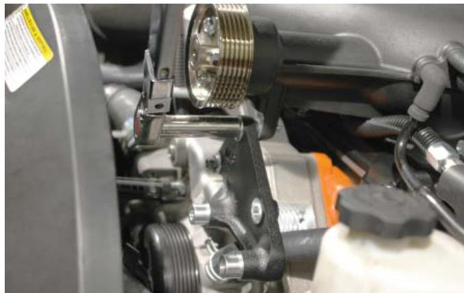
177. Add the idler pulley with the supplied longer bolt to incorporate the bracket brace installed earlier. Use a 15mm wrench and torque to 40 ft lbs.
