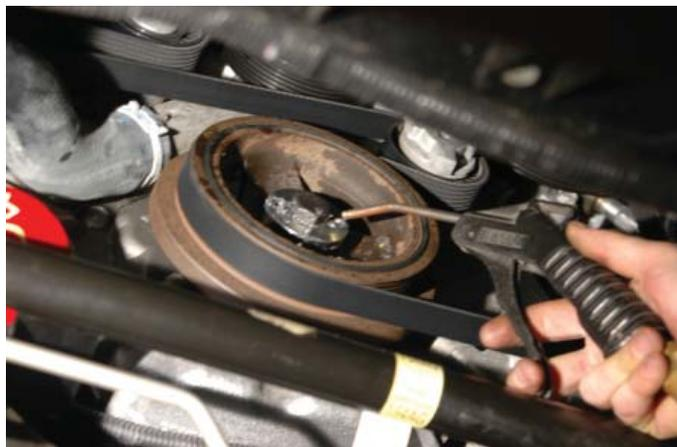
190. Ream out the two holes using the provided reaming bit.
