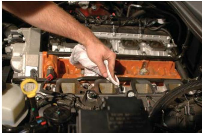
33. Use tape or shop rags to cover the exposed ports to prevent contamination.
