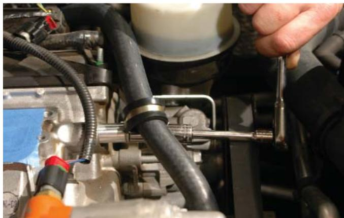
60. Route the hose over the power steering reservoir, between the dip stick and front coil pack, back around the remaining coil packs and cut to fit at the 90° elbow on the OEM heater hose. Secure in place with a supplied spring clamp.
