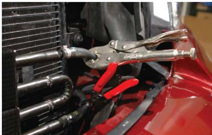
68. Use a drain pan to catch dripping fluid from the power steering cooler, and cut the two hose clamps holding the pinched hoses to the power steering cooler. Pull the hoses off the hose barbs of the power steering cooler, and pull the cooler off the plastic tabs mounting the cooler to the face of the air conditioning condenser. Set the power steering cooler aside for later reinstallation.
