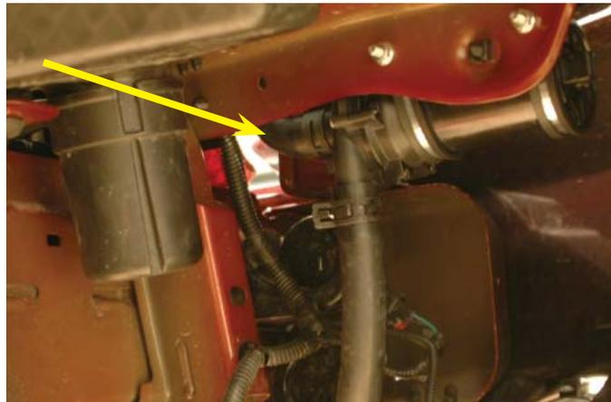
141. Remove the forward passenger side fuel rail mounting bolt using a 10mm wrench.
