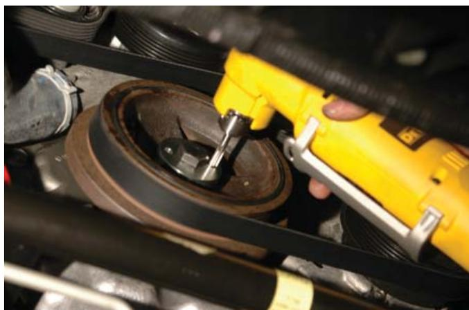
191. Remove the temporary crank pulley bolt and drill guide.
