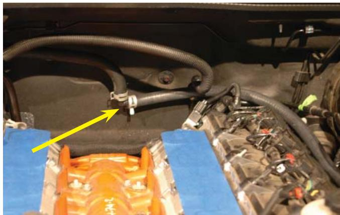
61. Cover the hose at chaffing points with the supplied split loom to protect the hose from damage.
