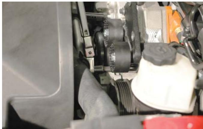
181. Tighten the OEM tensioner assembly back down using a 15mm wrench to 20 ft lbs.
