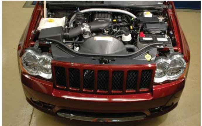
205. Test drive the vehicle for the first few miles under normal driving conditions. Listen for any noises, vibrations, engine miss fires or anything that does not seem normal. The supercharger does have a slight whining noise under boost conditions, this is normal. Also during the supercharger break-in, the rotors are self honing, the noise will reduce quickly.
