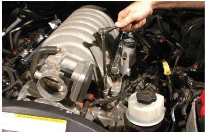
30. With the help of an assistant, carefully lift the OEM intake assembly from the vehicle. At this time if you didn't have success pulling the MAP sensor plug free, with the manifold moved slightly forward you should have an easier access to disconnect the sensor. Snake the brake booster hose around the existing water heater hoses as you pull the intake assembly out of the vehicle. Set aside as we will be using components later in assembly.
