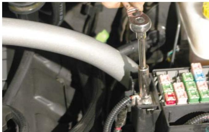
156. Remove the 25A fuse #43 for the coil-actuators from the rear fuse center. Verify using the owner's manual that you are removing the coil-actuators fuse. Do not rely on just the fuse number specified.
