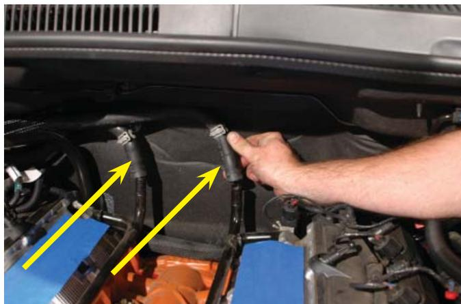
36. Use a 10mm wrench to remove the nuts holding the ground wires and ground sensor from the studs anchoring the heater hard lines to the back of the block. There are ground wires on both the driver side and passenger side. Pull these wires and the ground sensor from their studs.
