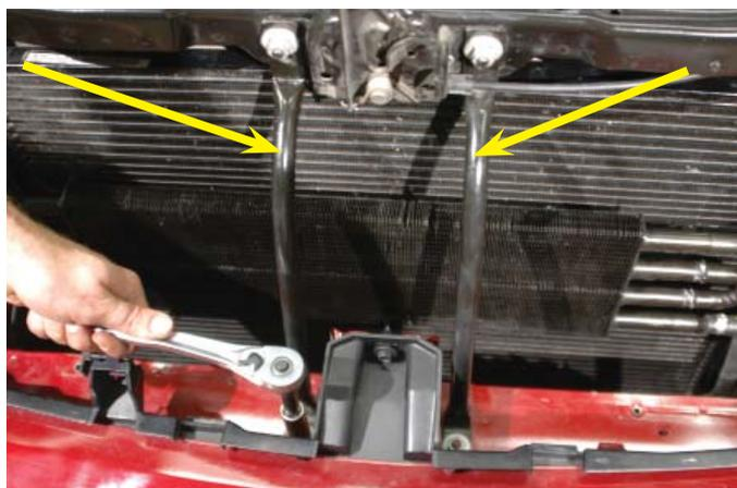
67. Use pinch off pliers or (carefully) vice grips to clamp off the two power steering hoses prior to the power steering cooler.
