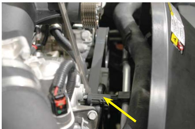
171. Use a 3/8" socket or breaker bar to spring the tensioner to remove the factory drive belt. We used a piece of pipe over a ratchet to gain leverage.
