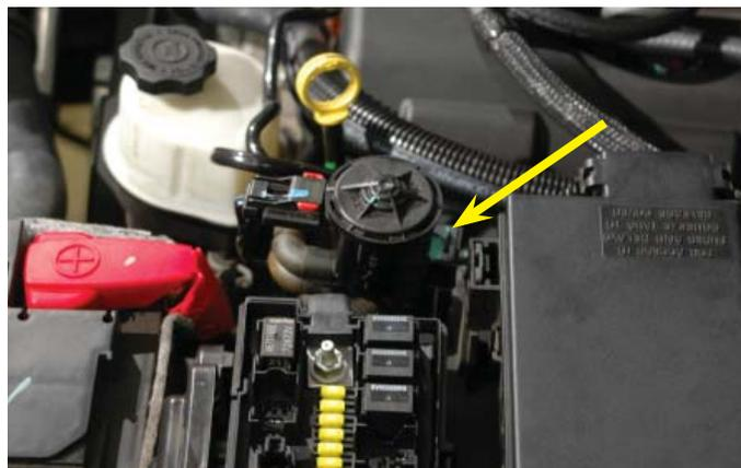
124. This is the intercooler pump and mounting hardware.
