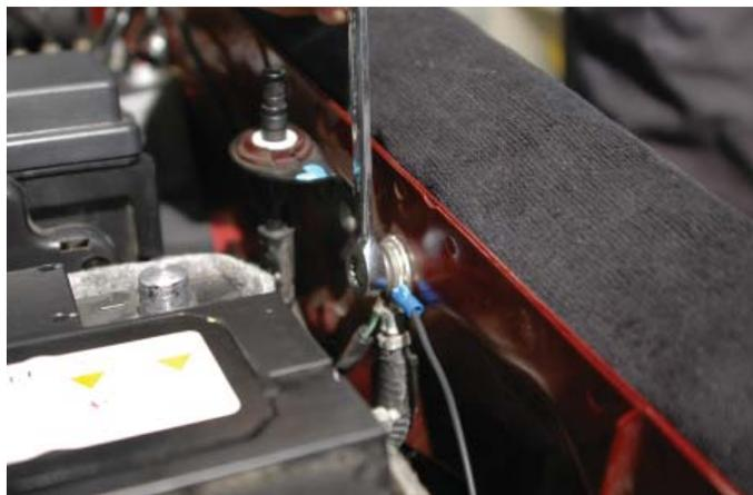
163. Cover the black ground wire with a length of the supplied split loom.
