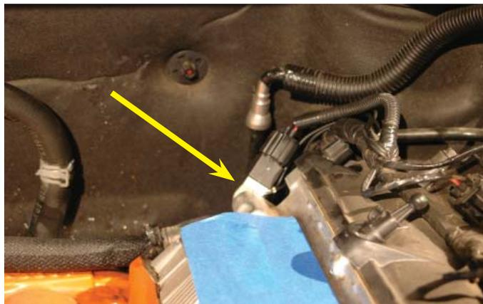
45. Replace the passenger side ground wires to the head using the original stud. Make sure you have accounted for all the wires.
