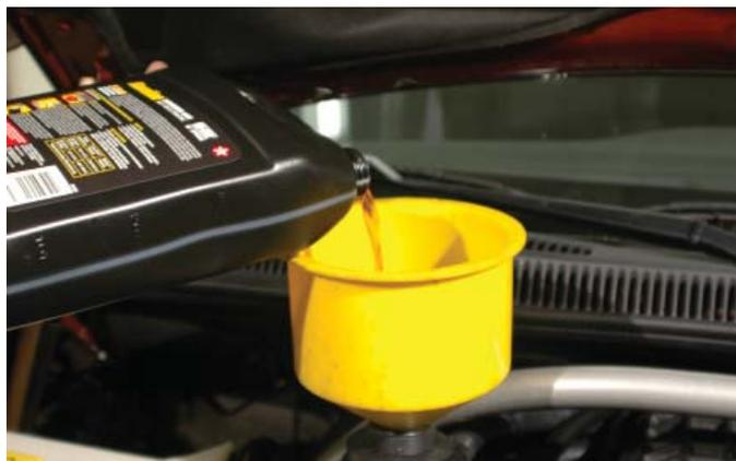
204. After the initial start up and the engine has come to operating temperature, recheck the coolant levels in the engine and intercooler reservoir. If necessary open the bleed valve again to allow any residual air trapped to escape the system. Check all the hose connections.
