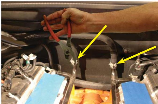
35. Disconnect the two heater hoses from the hard line barbs. There will likely be some residual coolant in the hoses and tubes, so take appropriate precaution and dispose of contaminated shop towels properly.
