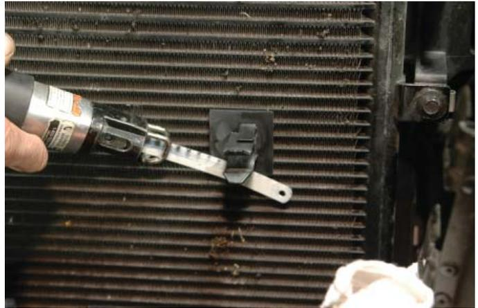
70. There is an existing threaded hole in the top surface of the bumper support on the driver side. Use a drill motor and drill bit to open this hole to 1/4".
