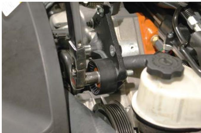
178. Add the supplied nut to the back of the idler pulley bolt securing the idler bracket brace using a 15mm wrench.
