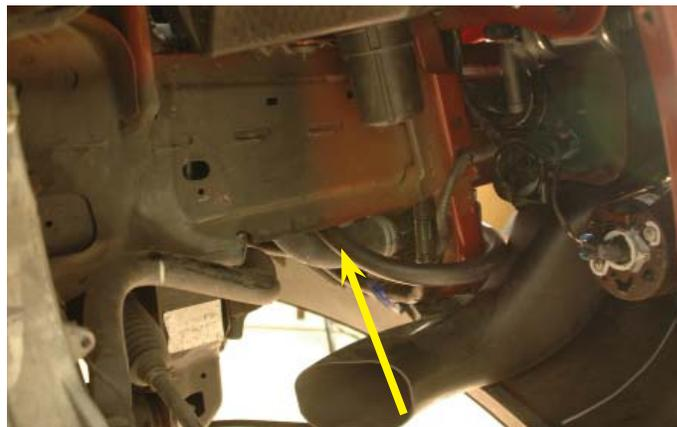
137. Connect the short end of the other modified 4" x 60" x 90° elbow hoses to the driver side hose barb of the intercooler heat exchanger and route over toward the passenger side to parallel the hose just installed into the wheel well. Secure in place with a provided spring clamp.
