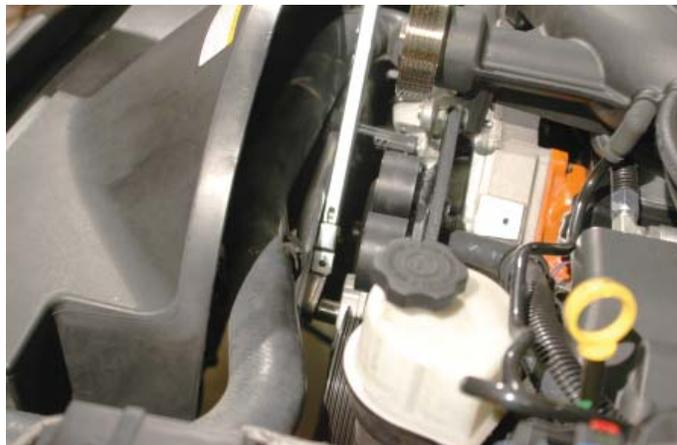
182. Install the drive belt on the engine using the belt routing diagram located on the last page of these instructions as a guide. Spring the tensioner using a 3/8" ratchet or breaker bar (we use a pipe for ease of leverage on a 3/8" ratchet).
