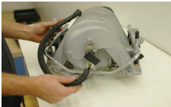
108. Remove the brake booster valve from the end of the hose and re-connect the valve to the opposite end of the hose by the "J" bend.
