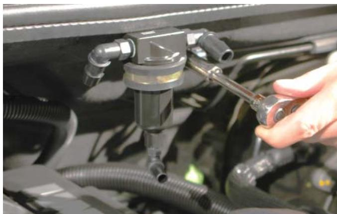
115. Trim the 3/8" hose to fit between the oil separator valve and oil fill spout barb and install between the two, no clamps are necessary.
