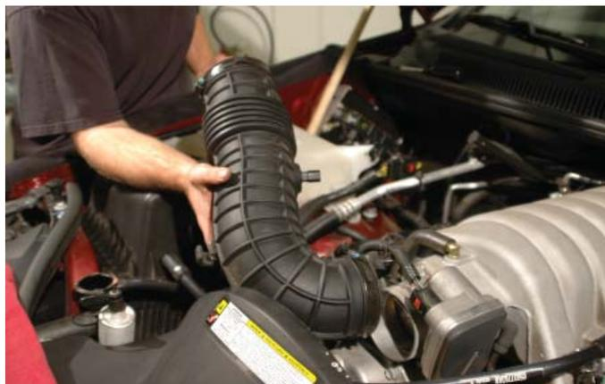
20. Pull the throttle body harness anchoring clip from the throttle body mounting bracket as shown.
