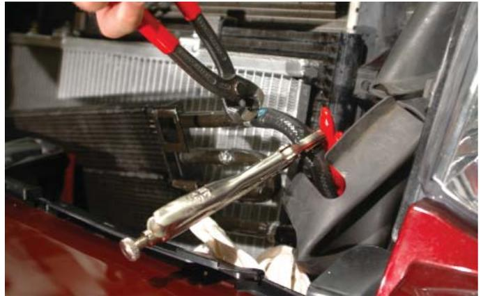
77. Remove the pinching pliers or vice grips from the two power steering cooler hoses. Attach the supplied acute (below 90°) angle mounting bracket to the passenger side, lower power steering bracket with the angle being up leg pointing forward. Use the supplied threaded plate as backing with the supplied bolt. Align the backing plate flush with the top of the bracket and tighten securely.
