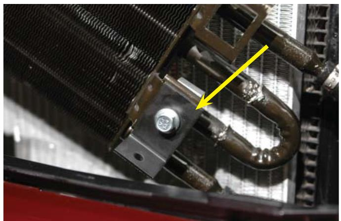
79. Use the provided bolts and nuts to attach the two mounting brackets to the two holes prepared in the top surface of the bumper support. Tighten the bolt and backing plate of the driver side mounting bracket.
