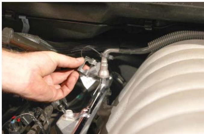
28. Use shop rags to catch residual fuel and the fuel line removal tool to disconnect the fuel line from the passenger side fuel rail. First press the fuel line further onto the fuel rail barb, then push the fuel line removal tool into the fuel line to release the locking clip. Now pull the fuel line free. We recommend plugging the fuel line and capping the fuel rail barb. Clean up residual fuel using shop rags and dispose of the contaminated rags properly.
