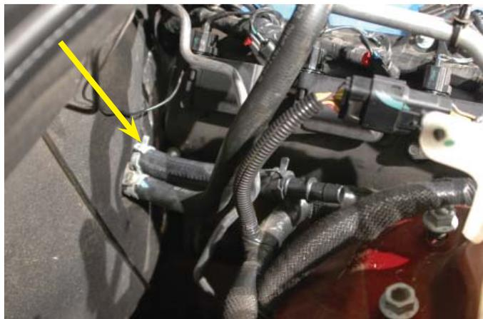
54. Cut the passenger side hose installed at the water pump to meet the coupling (hose mender) installed on the 7" hose just installed. Press onto the coupling and secure with a supplied spring clamp.
