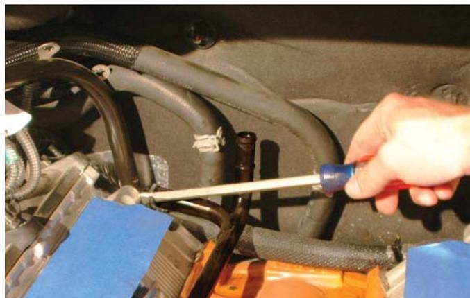
44. Replace the driver side ground sensor and ground wires to the head using the original stud. Clock the ground sensor toward the driver fender to gain the clearance necessary for the supercharger installation.
