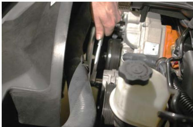
174. Going clockwise (toward the driver side) from the first water pump bolt, skip one, then using a 13mm wrench remove the next bolt. You may need to rotate the tensioner assembly to pull the bolt free.
