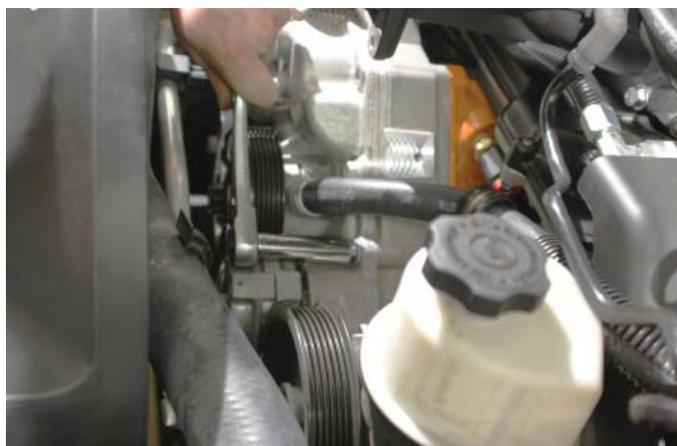
175. Replace the second water pump bolt (you just removed) incorporating the supplied idler bracket as shown. Finger-tighten the bolt at this time.
