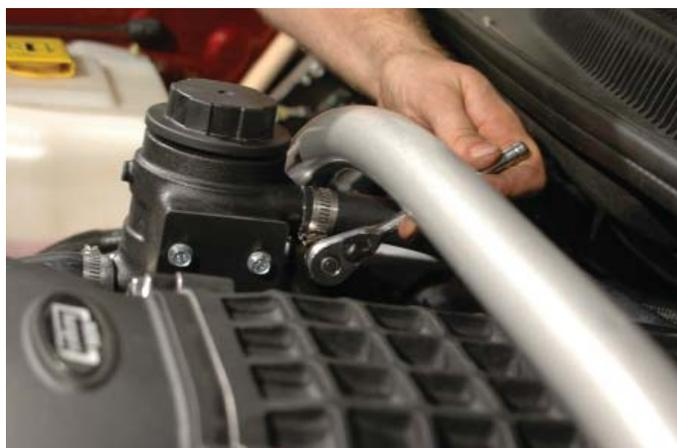
147. Connect the hose from the driver side barb of the supercharger intercooler to meet the hose from the intercooler pump inlet barb. Cut the hoses to fit and connect together using the provided coupling (hose mender), and secure in place using the provided spring clamps.
