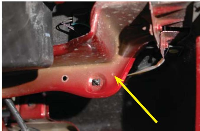
130. Drill a  $\frac{1}{4}$ " hole at the mark for an intercooler pump mounting clamp.
