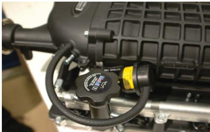
85. Remove the throttle body from the OEM intake manifold assembly using a 10mm wrench.
