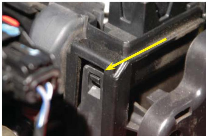
10. Lift the forward fuse center and unplug the two wire harness plugs from the bottom of the fuse center. Pull the fuse center up and over toward the engine.
