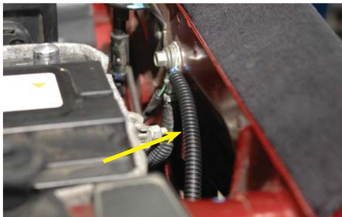
164. Replace the fender well splash shield on the passenger side using the removed plastic push rivets and removed plastic “pop” rivets where you have access to both sides. In this case push the locking pin back into the hole of the ‘pop’ rivet locking it in place. Where you don’t have access to both sides use the provided push rivets.
