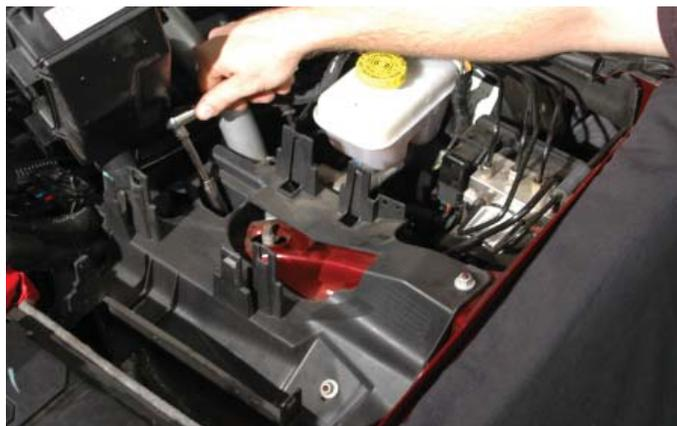
120. Re-connect the two forward fuse center plug connections.
