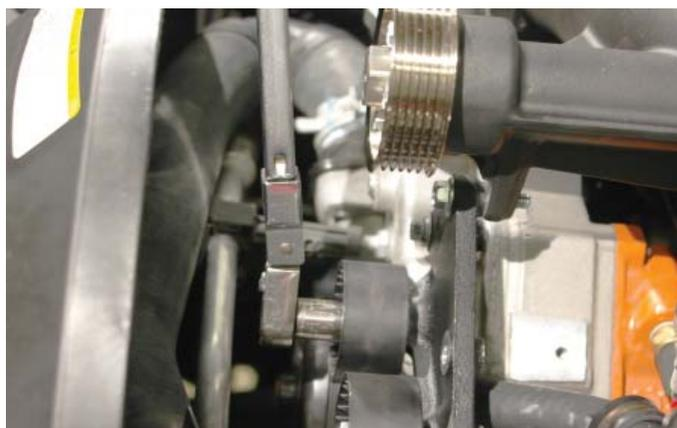
180. Torque the second water pump bolt (finger-tightened earlier) using a 13mm wrench and torque to 20 ft lbs. Always verify your torque wrench settings.
