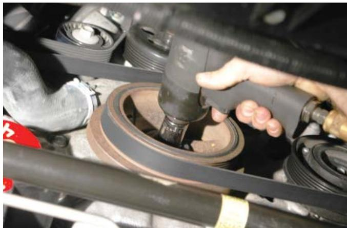
187. Install the provided drill guide using the provided crank bolt and torque to 40 ft lbs. It's helpful to align the holes in the guide horizontally.
