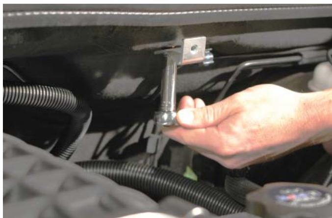
114. Use the provided Adel clamp and bolt to attach the oil separator to the bracket just installed using a 10mm wrench. The embossed arrow on the top of the valve points toward the driver side fender. Once installed, twist the driver side barb to point down and the bottom barb to point toward the oil fill spout.
