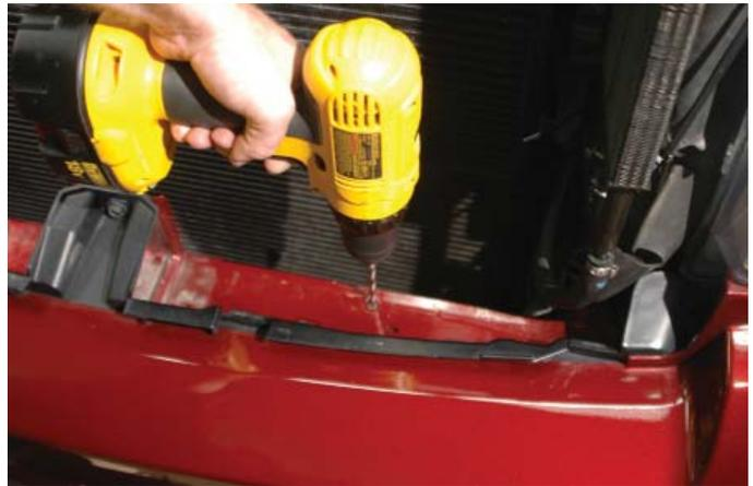
71. Measure over 19" toward the passenger side, mark and drill another 1/4" hole to match the setback of the existing hole.
