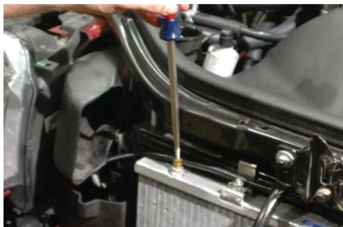
199. Fill the radiator back up with the fluid drained earlier. Be sure to incorporate a filter in case any debris contaminated your fluid. Top off as necessary.
