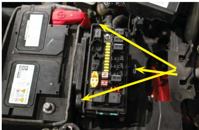
122. Replace the rear fuse center on the four fuse center mounting bracket posts. Ensure they click into place.
