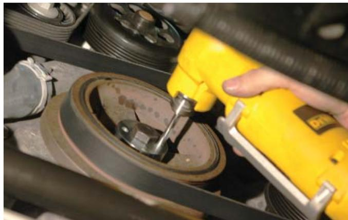
189. Blow out the holes using compressed air. Wear safety glasses.
