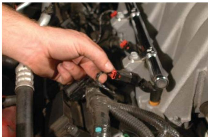
23. Disconnect the MAP sensor from behind the air intake manifold on the passenger side behind the OEM manifold. If you cannot get this unplugged easily, you will have another chance while you are removing the OEM manifold a little later in the instructions.
