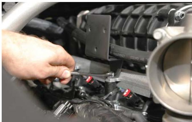
143. Modify the OEM passenger side coil pack cover to create clearance with the throttle body, slide under the intercooler reservoir mounting bracket and press onto the mounting studs locking in place.
