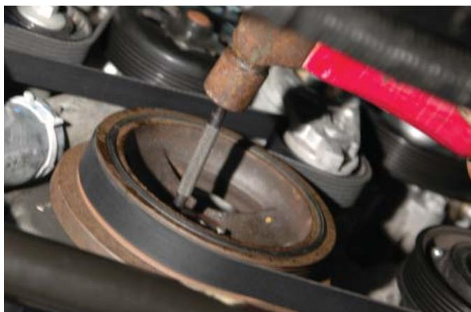
195. Install the OEM crank pulley bolt and torque to 129 ft lbs.
