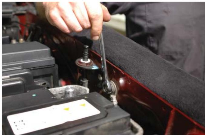
162. Route the black wire from the relay harness over toward the ground bolt. The existing "eye" terminal is not large enough to fit over the ground bolt. Cut the "eye" terminal off, strip off 3/8" of insulation from the end and crimp on the new "eye" and crimp on securely. Replace the ground wires and bolt incorporating the new black ground wire from the relay harness. **Ensure that you have ALL the ground wires attached.**
