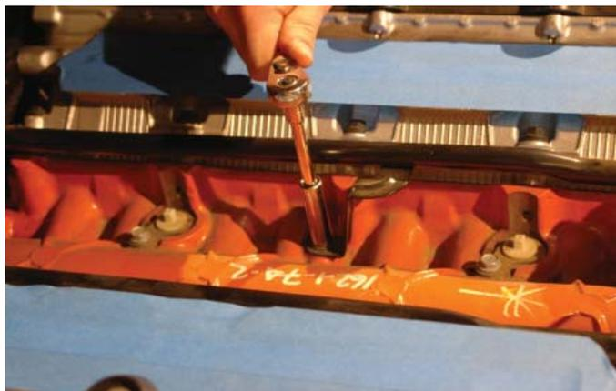
40. Use a 10mm wrench to remove the heater hard line mounting bolt from the water pump.
