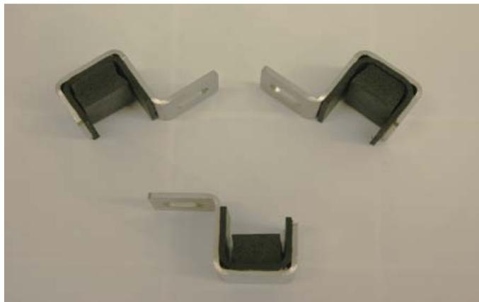
65. Use acetone or lacquer thinner to clean the end caps of the heat exchanger on the inside surface (the side opposite the hose barbs). Cut strips of the supplied adhesive backed foam to fit, and attach to the cleaned surfaces. This should completely cover the tanks and act as a buffer against the existing heat exchanger.
