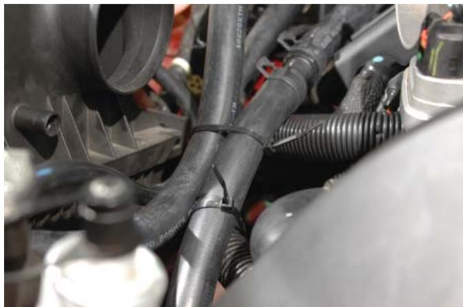
150. This is the intercooler pump relay harness. Install the provided 15A fuse in the fuse holder of the harness and replace the fuse cap.
