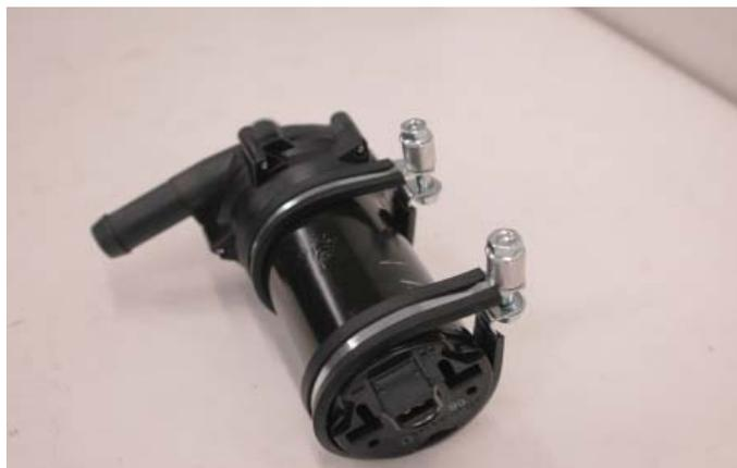
132. Secure the pump as described using the supplied nuts on the rear side of the fender cross brace. The discharge barb of the pump is to point down with the inlet barb of the pump pointing toward the driver side of the vehicle. Tighten in place using a 10mm wrench.
