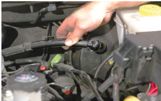
25. Disconnect the PCV vent tube running from the intake air box to the oil fill spout. Set aside for use in a later step.
