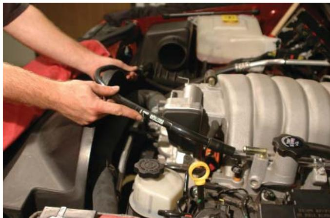
26. Disconnect the EVAP hose from the driver side of the manifold, just behind the throttle body.
