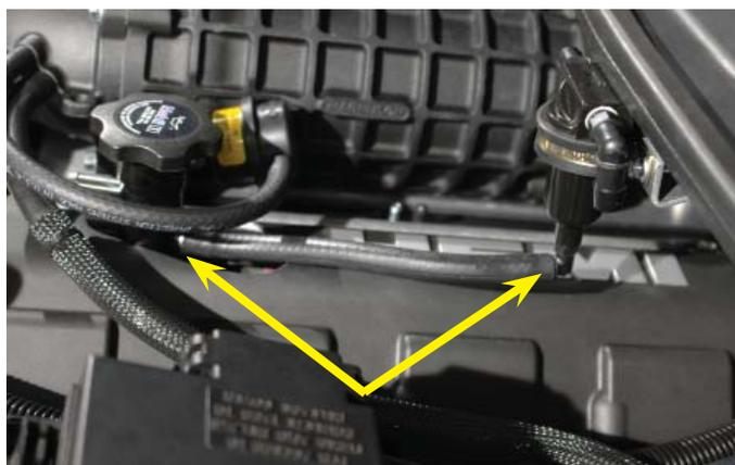
116. Install a 24" piece of the supplied 1/2" hose between the passenger side PCV barb in the supercharger lid and the passenger side barb of the oil separator valve.
