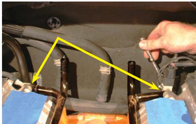
37. There are two zip-tie clamps holding the wire harness to the heater hard line mounting brackets. Cut these zip-ties off the brackets.
