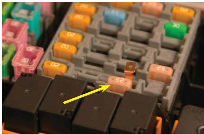
159. Strip 3/8" of insulation from the end of the yellow wire and crimp on the supplied spade connection.
