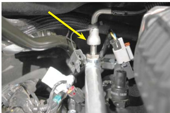
111. Pull on the fuel line; this should not be removable without using the fuel line removal tool. After verifying your connection, snap on the fuel line safety clip.
