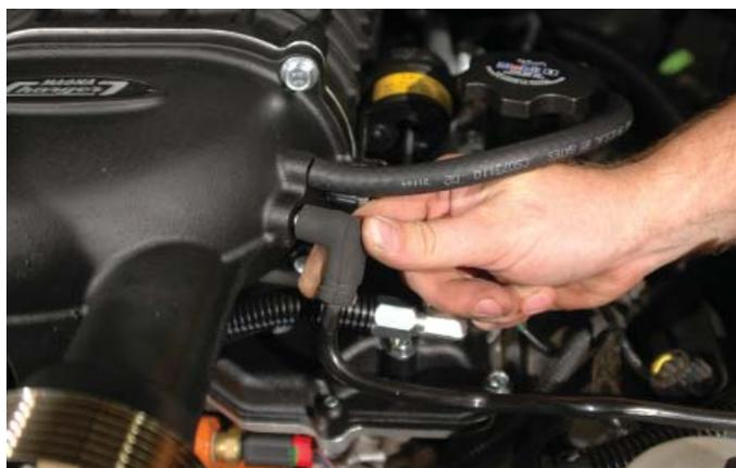
107. Remove the stock brake booster hose from the OEM intake manifold.
