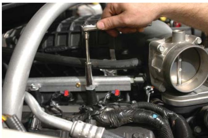
142. Attach the supplied intercooler reservoir mounting bracket to the forward passenger side fuel rail mounting boss location, re-installing the fuel rail mounting bolt. Tighten securely using a 10mm wrench.
