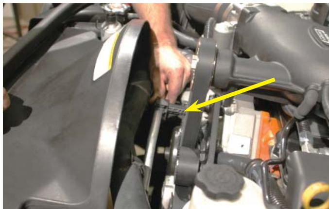
184. Remove the air box end of the hose from the OEM PCV plastic line and replace with the provided 4" section of 5/8" hose. Connect the remaining OEM hose end to the front oil fill spout hose barb and the new hose end to the air box end and air box. Secure to the air box using the provided spring clamp.
