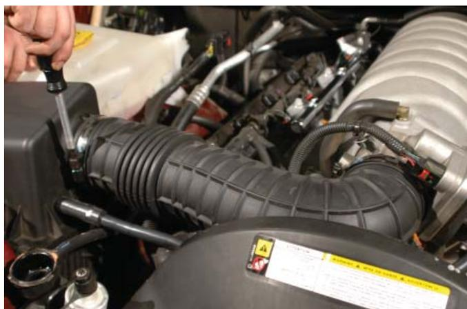
19. Remove the intake air tube from the vehicle. This will not be reused. There is a PCV vent tube running from the air box to the oil fill spout, this has a soft mounting clip on the intake air tube. Be careful to not damage the PCV vent tube.
