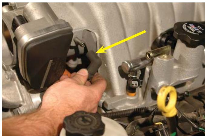
27. Remove the fuel line safety clip. Set aside for later.
