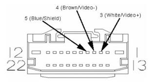
Figure 7: 22-pin Connector face
