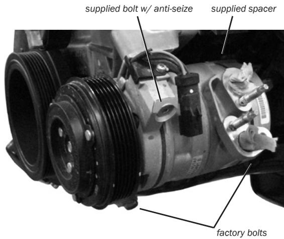
14. Install the starter (torque to 40 ft/lbs), modified A/C compressor (torque to 18 ft/lbs), and the engine idler pulley (torque to 40 ft/lbs).
