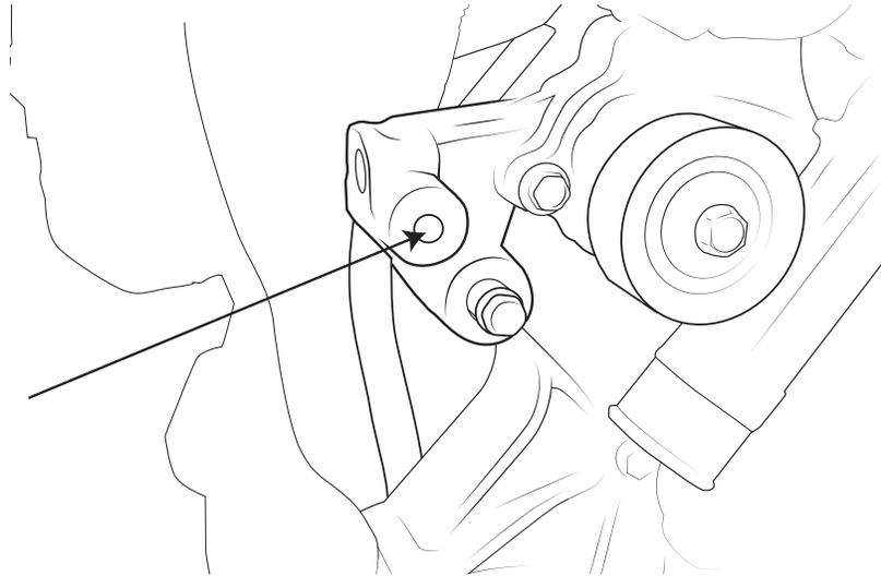
*Figure 22: Drill out upper alternator mounting hole.*
