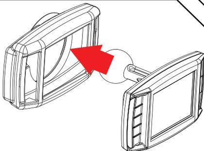
If using Bully Dog's available Ram Mount T-Slot Adapter (30600-3), slide the adapter into position on the device, and then insert the ball end of the adapter through the circular hole in the back side of the Armor.
