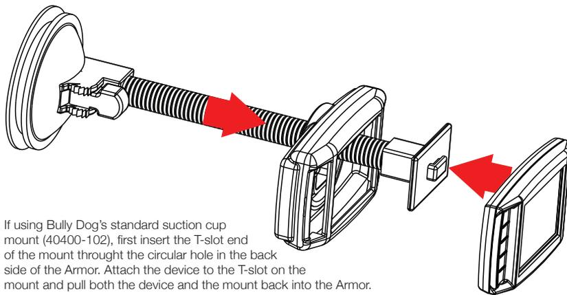
If using Bully Dog's standard suction cup mount (40400-102), first insert the T-slot end of the mount through the circular hole in the back side of the Armor. Attach the device to the T-slot on the mount and pull both the device and the mount back into the Armor.
