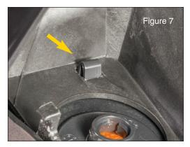
locate the tab on the top of the side marker light (Fig 7). Push the tab down to release the Side Marker light Assembly. Remove the assembly from the fender. Insert the driver Side Marker light Euro-Guard into the open fender
