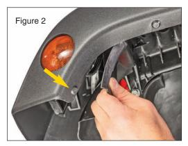
on the fender (Fig 2 & Fig3). Then locate the plastic rivet that holds the fender to the light housing located at the end of the fender lip (Fig4). **Use caution to** avoid any pinching of your fingers.
