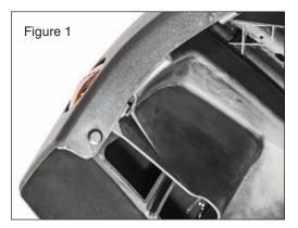
Put on safety glasses. First, Locate the front of the driver side inner fender well liner directly under the side marker light (Fig 1). Grab the front portion of the fender liner and pull it out over the tab
