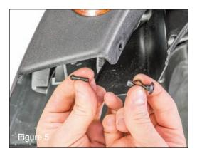
With a small allen wrench or punch, firmly push in the center of the plastic rivet. Note: It will take some force to push this center of the rivet through (Fig 4).
