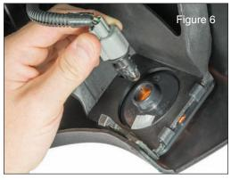
liner to locate the bulb assembly (Fig6). With the inner fender liner pulled back, remove the bulb assembly by twisting one quarter turn and pulling, unlocking it from the Side Marker Housing (Fig 6). With the light bulb assembly removed,
