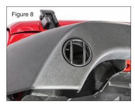
flare from the back side of the flare. The Euro-guard bars should be in the vertical position (Fig 8). Re-install the Side Marker Light into the fender wedging the Euro-Guard into the fender (Fig 9). The Side marker housing should "click" into place.
