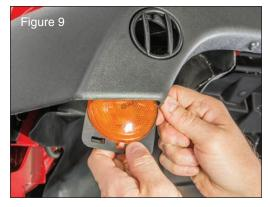
With the Side Marker Light Assembly and bulb assembly installed, push the fender liner assembly back over the plastic rivet head by using the removed Rivet and secure in place. Re-install the inner fender liner and secure the plastic rivet. (Reversing the removal procedure in early steps).
