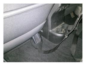
On the 4 dr unlimited wrap the strap around the inside seat bracket first and then to the outside foot and back upto the net
