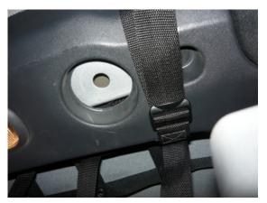
The two straps that run out horizontilly at the top go over top the roll bar and come out around the side. These connect into the cam buckles on the net. (see Photo). Tighten up both sides and postion the net so everything is centered and hanging evenly
