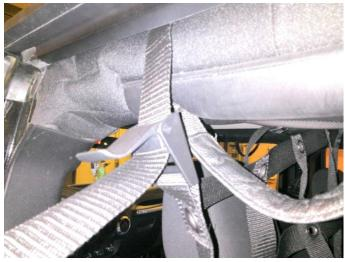
The long straps at the bottom pull down and wrap underneath the front seat seat brackets as shown. The JK and JKU have different style seat brackets. As seen in the two photos. The straps come back up and connect into the lower Cam buckle.
