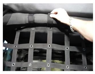
Look at the photos to see how it is positioned along the roll bar. The outermost straps on either endwraps around the roll bar on the opposite side of the roll bar.
