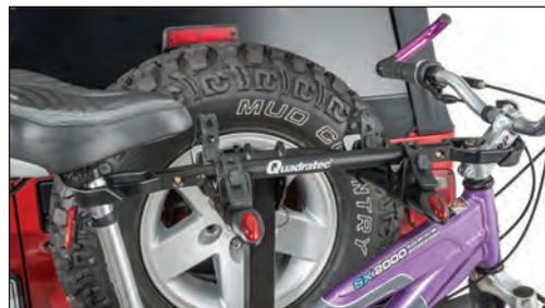
*Adapter takes the place of a traditional top tube, allowing standard bicycle rack installation.*
