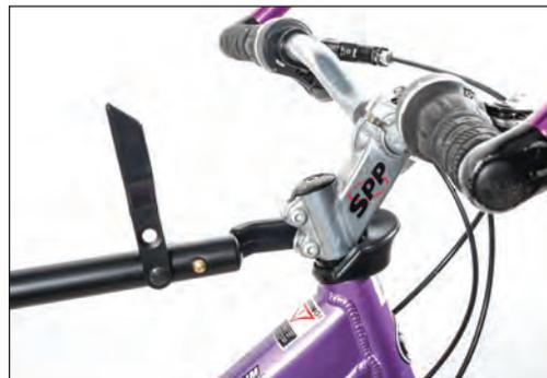
*Slide the adapter to correct length for your bicycle. Place the larger collar around the handlebar stem of the bike.*
