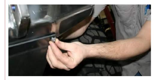
${\bf 5}~$  To install the bolts near the lights, you will need reach through the light hole as shown below.
