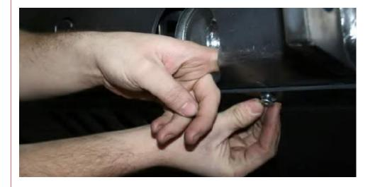
6 The easiest way to install the middle bumper bolt is to reach up and around the lower crash bar. You may also try and reach through the slot in the skid.
