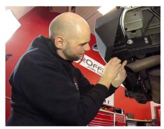
11. Next, using a 1/2 drill bit, drill a hole into the passenger lower mounting hole into the lower cross member. Once this is done, loosely install the two (2) half inch bolts into the lower cross member.
