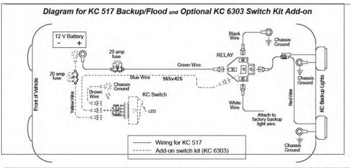
10. Below is a wiring diagram that can be used for powering the back-up lights.
