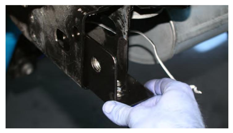
6. If installing the optional Fog Lights, bolt the lights into the brackets welded into the top back side of the bumper. Use the hardware provided with the fog light kit.
