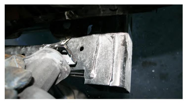
2. The body mounts should be the last part holding the crossmember to the frame. Once they are cut, you should be able to remove the back section and discard.
