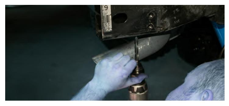
4. Once the holes have been drilled, be sure to apply paint to the exposed metal.
