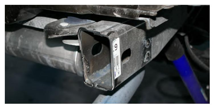
3. Apply primer and paint to the exposed cut areas and allow to dry.
