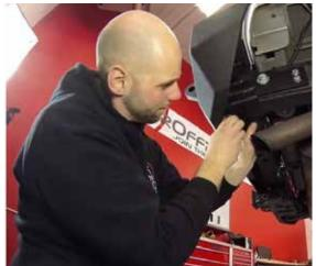
Next, using a 1/2" drill bit, drill a hole into the passenger lower mounting hole into the lower cross member. Once this is done, loosely install the two (2) 1/2" bolts into the lower cross member.
