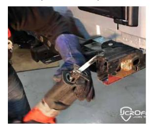
4 Next, print the JK rear bumper installation template PDF file by clicking the link or you can find it on our website under install instructions. Cut out the drillingtemplate and put them on the bottom of the frame.
