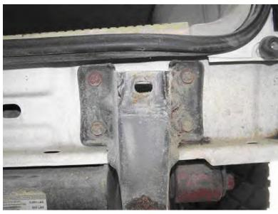
Remove the factory rear bumper. There are two mounting brackets attaching the bumper to the back of the bulkhead with 4 bolts each.
