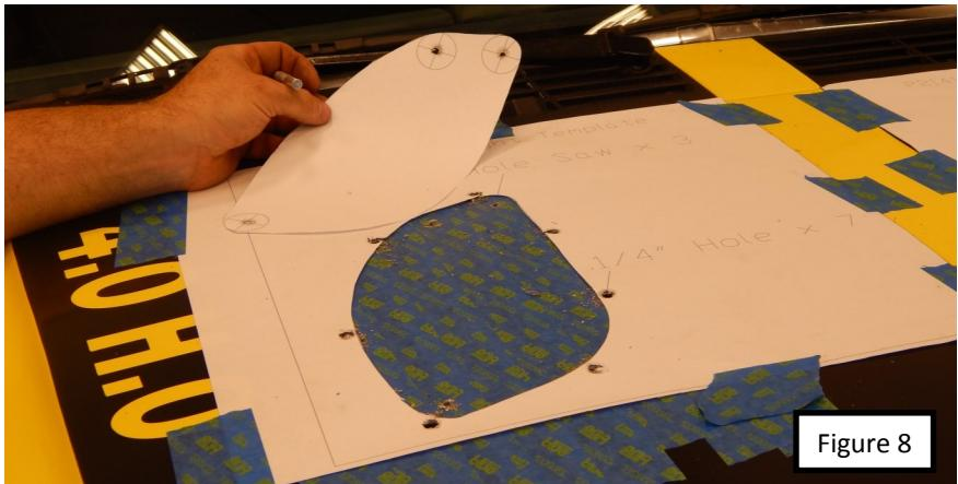
10. Trace the perimeter of the vent cut out on to the hood (Figure 9).
