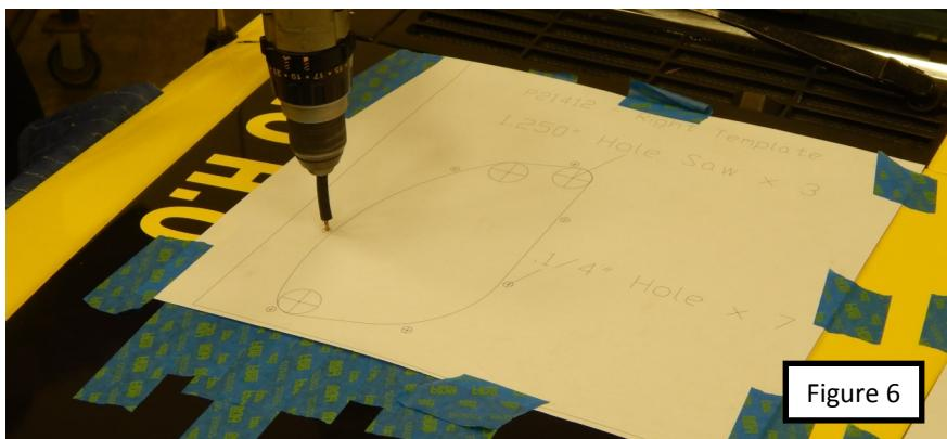
8. Open up the 14 holes (7 per side) on the perimeter of the hood vent cut out to 1/4" (Figure 7).
