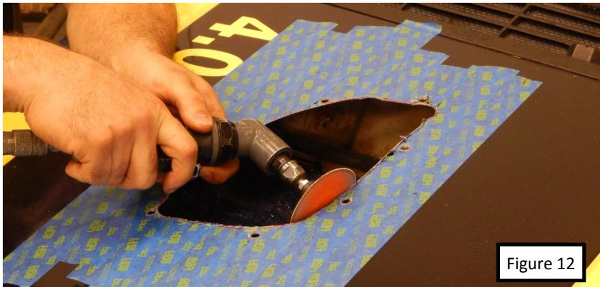
15. Ensure the hood vent has a bit of wiggle room. This will make for a smoother final installation.
