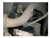
2) Using a hacksaw or sawsall, cut the stock tailpipe off where it exits the muffler. (This step is not mandatory, but it makes removal a little easier.)
