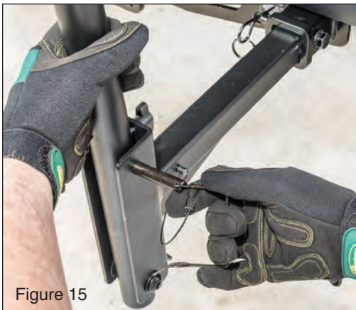
In order to recline the bike rack and gain access to your tailgate or cargo area, start by removing the bicycles from the rack. Lower the upper arm using by removing the retaining pins and re-installing them in the upper holes.
