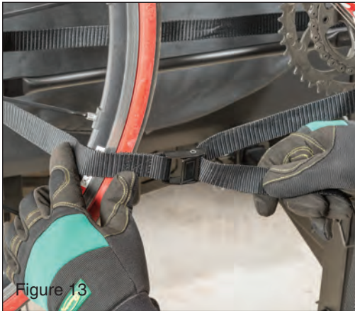
Thread the provided safety strap through the wheels and the back of the vertical arms of the rack. Secure with
