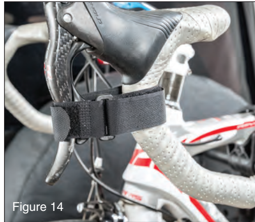
the buckle (FIG 13). Hook & loop straps can be used to secure brakes to prevent wheels from spinning in transit. (FIG 14)
