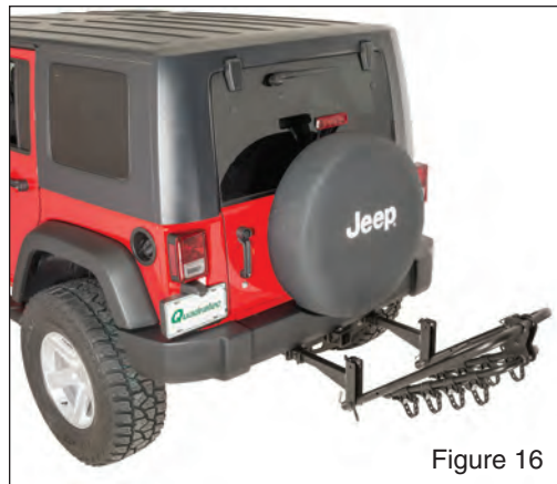
Now remove the retaining pins from the lower hinges and carefully recline the main rack. Be sure to reinstall all pins and retaining clips when you are finished and before operating your vehicle.
