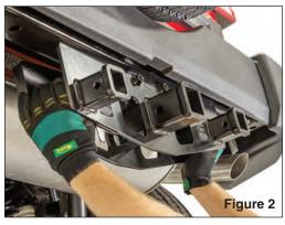
Install the Versahitch over the rear cross member, then install the 4 supplied bolts through the hitch and rear cross member and thread them into the weld nuts on the Versahitch.
