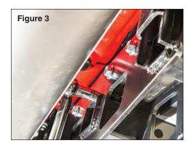
Torque the bolts to 80 ft.lbs. using an 18mm socket and a torque wrench.
