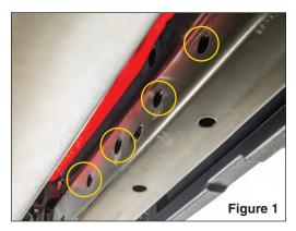
Put on safety glasses. Locate the four bolt holes in the rear cross member of your vehicle behind the Rear bumper.
