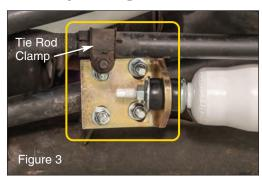
Pull the stabilizer shaft exactly half way out. Stabilizer must be kept out exactly half way (4.1875") during installation. Mount stabilizer to track bar (see FIG 3) and tie rod (see FIG 4).
