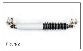
the stem bushings, washers and nuts. (see FIG 2) Install nuts using a 14mm socket, loosely at this time. Make sure the stem bushing lips are towards the mounting hole in the brackets.
