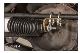
Install 1.25" U-Bolts around track bar and 1" U-Bolts around tie rod using flat washers and nylock nuts using a 1/2" socket, but do not tighten yet.
