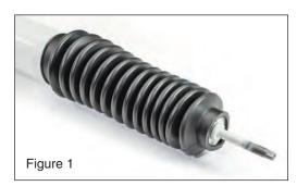
Install supplied boot over secondary stabilizer and secure using the boot tie. Install the secondary stabilizer brackets loosely onto each end of stabilizer using
