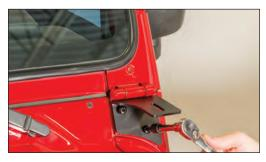
Tighten the bolts with a T40 Torx bit and ratchet. Install the light on bracket as shown and tighten the hardware.
