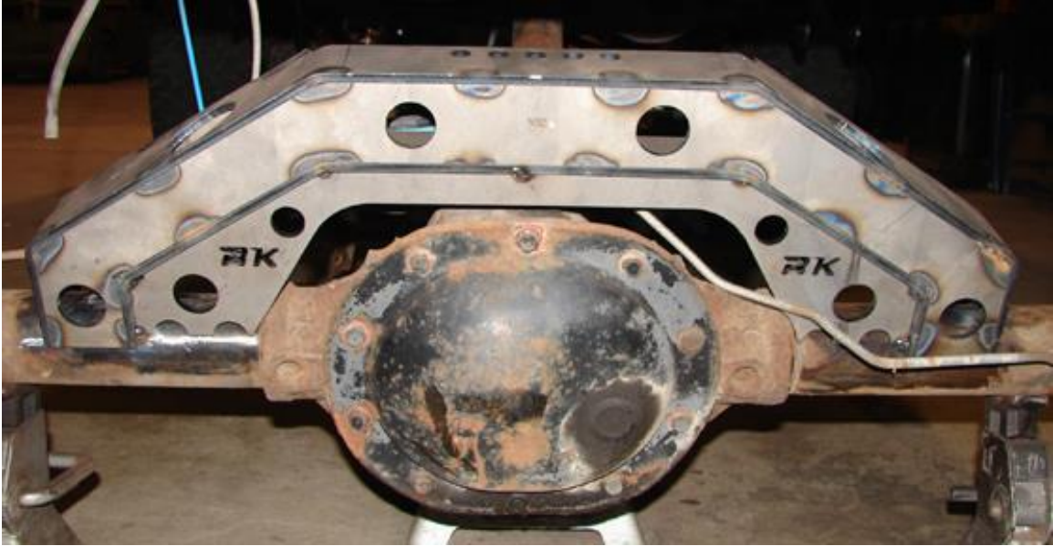
Cradle Tie in Plate Installed
