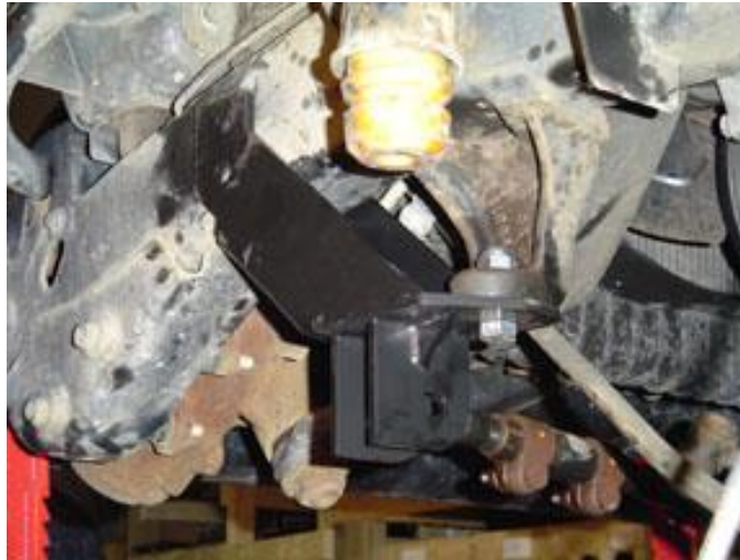
Track Bar Bracket Installed
