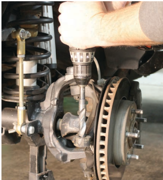
Drilling out knuckle to 18mm
