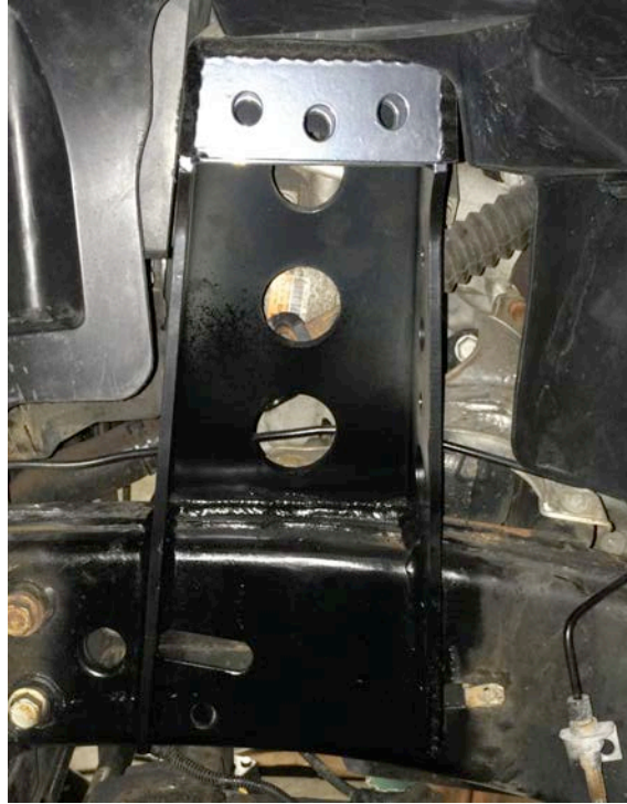
Front Upper Coil Over Mount Positioned on the Frame
