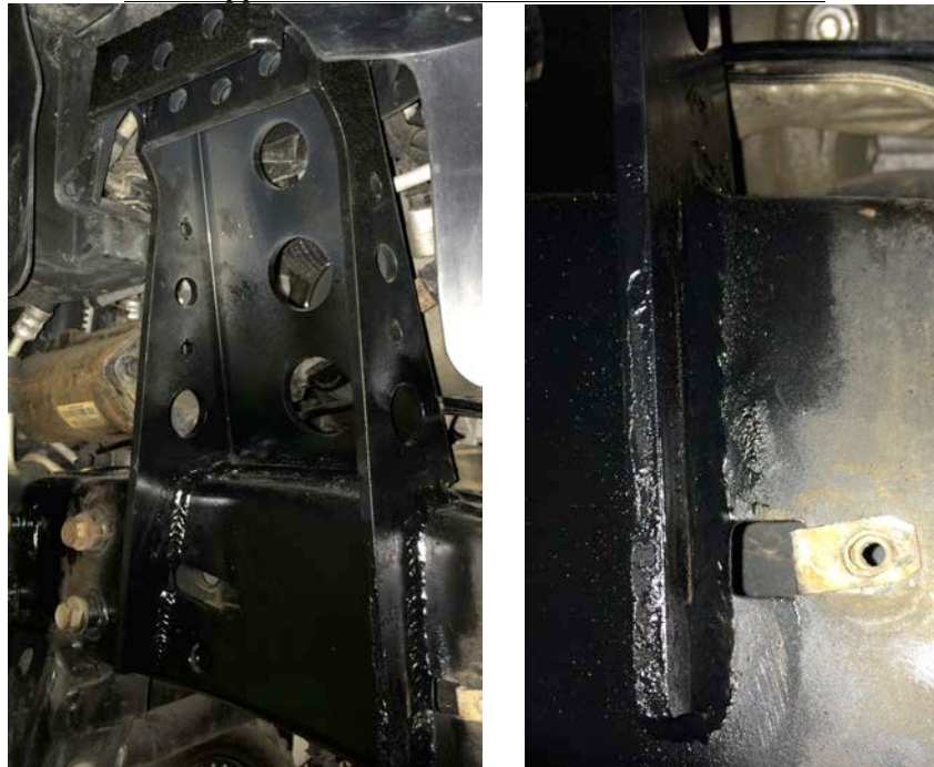
Front Upper Coil Over Shock Mount Welded to the Frame
